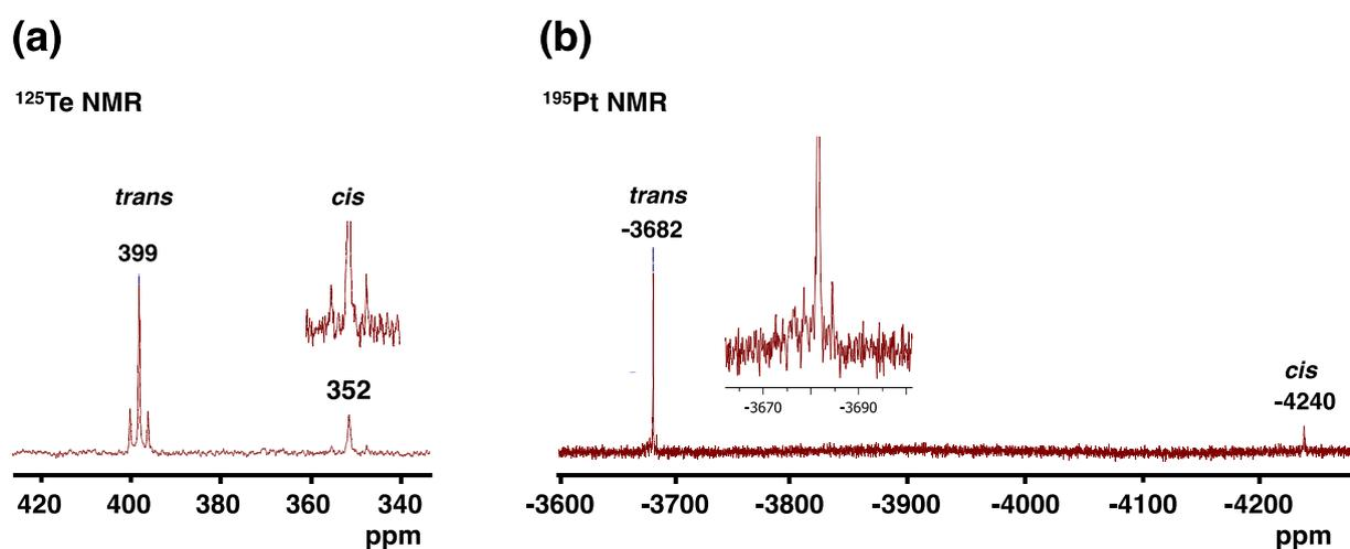
Figure 1. (a) The  $^{125}\text{Te}\{^1\text{H}\}$  and (b) the  $^{195}\text{Pt}\{^1\text{H}\}$  NMR spectra of the mixture of the *cis*- and *trans*-isomers of  $[\text{PtCl}_2\{\text{Te}(\text{CH}_2)_6\}_2]$ .
