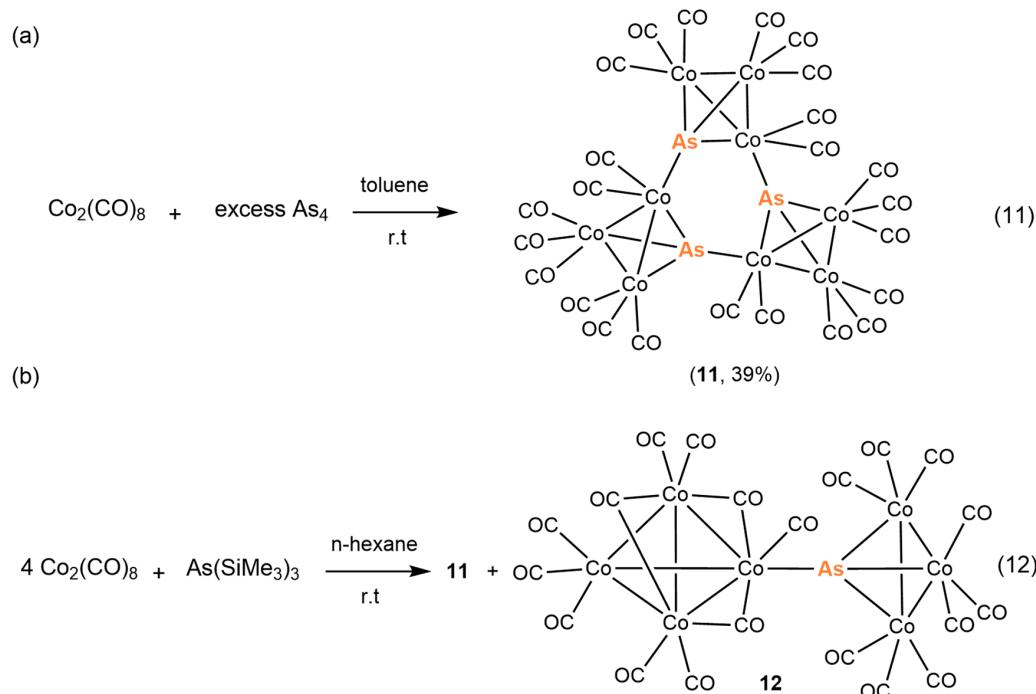
**Scheme 5.** Synthesis of the cyclic clusters (**a**) **11** from the reaction of  $\text{Co}_2(\text{CO})_8$  with  $\text{As}_4$  in toluene at room temperature (Equation (11)), and (**b**) **12** from the reaction of  $\text{Co}_2(\text{CO})_8$  with  $\text{As}(\text{SiMe}_3)_3$  in  $n\text{-hexane}$  at room temperature (Equation (12)).
