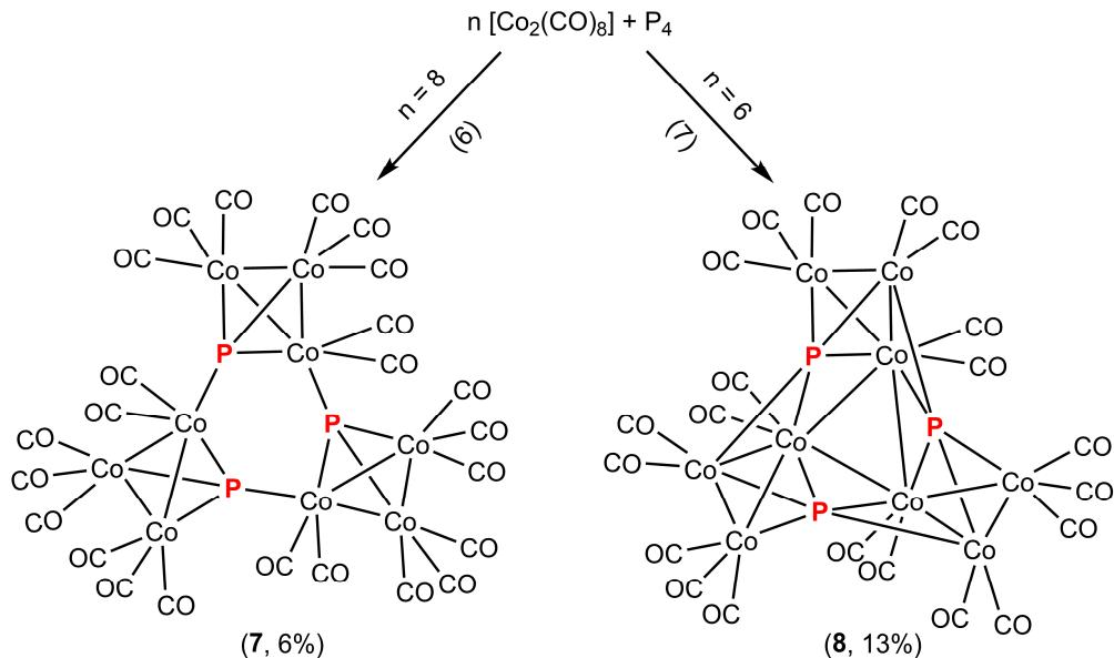
**Scheme 3.** Synthesis of the cyclic clusters **7** and **8** from the reaction of  $P_4$  with eight eq. of  $Co_2(CO)_8$  in toluene at room temperature (Equation (6)) and six eq. of  $Co_2(CO)_8$  in hexane at room temperature (Equation (7)), respectively.
