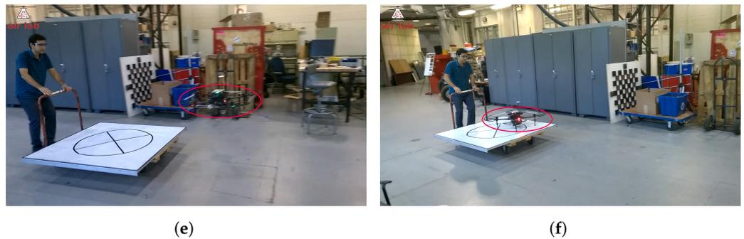
**Figure 7.** (a–f) Screenshots from a video sequence showing our quadrotor landing on a moving platform. In this experiment, the quadrotor is additionally equipped with a DJI Guidance sensor for safe operation in the indoor environment.
