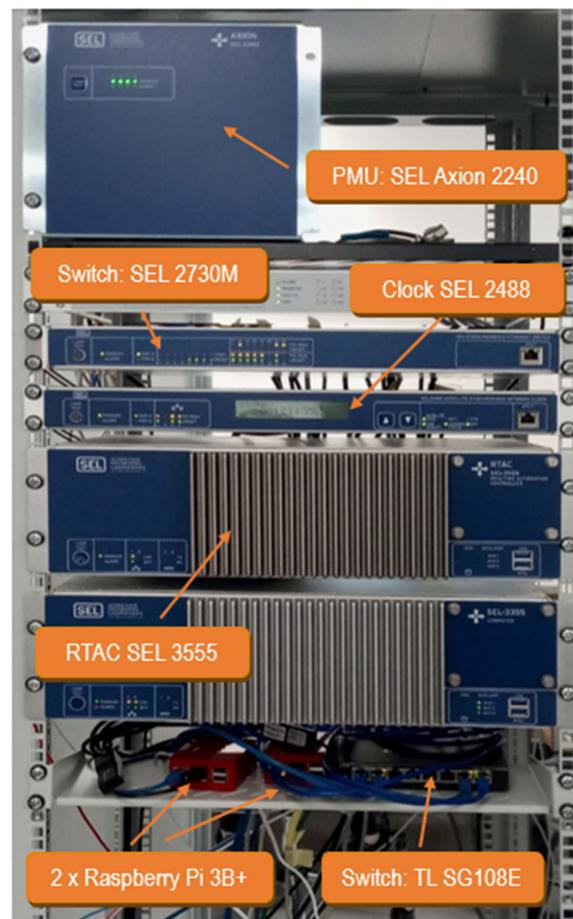
**Figure 4.** Laboratory testbed (RTDS not shown).
