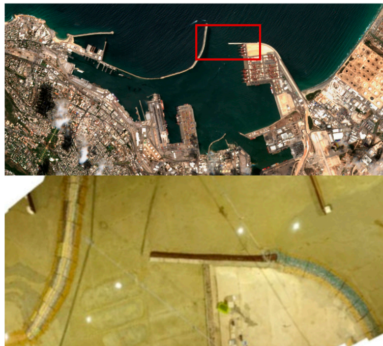
Figure 1. Aerial imagery for oil spill simulation. The top image depicts a satellite view of the Haifa Port, with a highlighted red rectangle indicating the focus area. Below is a stitched image of a scaled-down model (1:120 ratio) of the same section of the port, recreated in a controlled pool environment.
