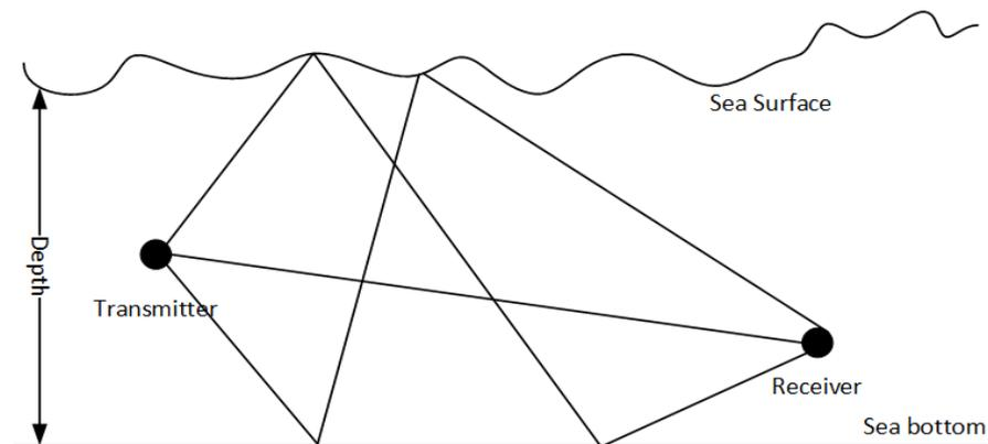
**Figure 10.** Model of shallow UWA multipath channel.
