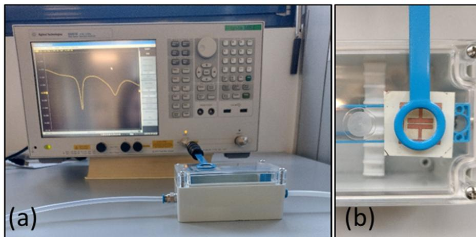
**Figure 2.** Set-up used for the measurements. (a) Measurement configuration showing the circular antenna probe connected to the vector network analyzer above the measurement chamber where the humidity is controlled. (b) Detailed image of the measurement chamber, showing the probe outside the chamber and the sensor inside the chamber.
