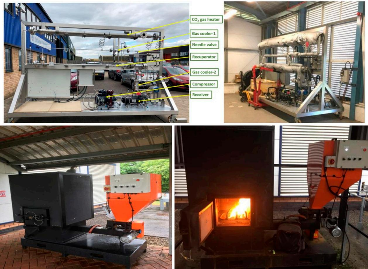
**Figure 11.** A small-scale power generation and heat recovery test rig based on biomass with CO<sub>2</sub> transcritical Brayton cycle [64].
