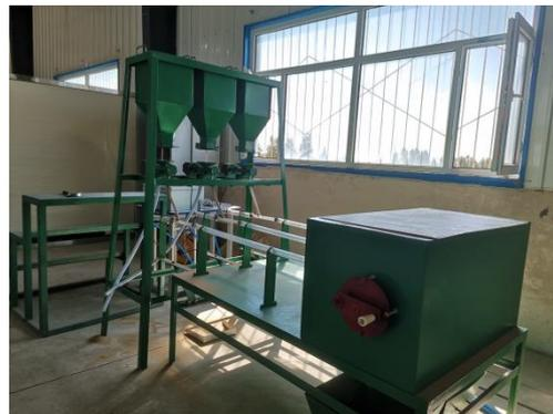
Figure 3. Test equipment of wind turbine blade erosion device.
