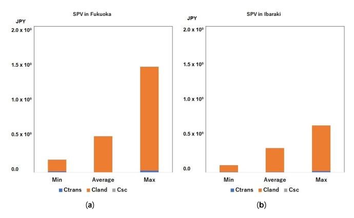
**Figure 13.** Comparison of the cost factors in  $C_{loc}$  for SPV in (a) Fukuoka and (b) Ibaraki simulation areas, with the minimum, maximum and average values across the 500  $\times$  500 simulation area points.
