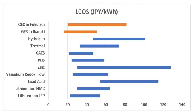
**Figure 17.** Comparison of the LCOS of GES in the simulated SPV-GES hybrid cases with the LCOS benchmarks of other energy storage technologies in Japan [benchmark data obtained from].
