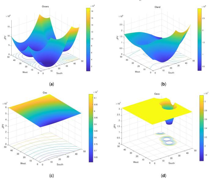
**Figure 7.** The GES location-dependent cost variations in the  $500 \times 500$  Ibaraki suburban simulation area for (a) transmission (10<sup>7</sup>), (b) land (10<sup>6</sup>), (c) supply chain (10<sup>7</sup>) and (d) excavation (10<sup>7</sup>).
