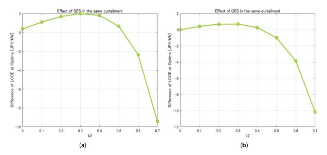
**Figure 19.** The variation of the LCOE difference between a SPV system and a SPV-GES hybrid system at the cost-optimized locations in (a) Fukuoka and (b) Ibaraki simulation areas with curtailment rate (positive values indicate LCOE has increased due to the introduction of GES; negative values indicate LCOE has decreased due to the introduction of GES).
