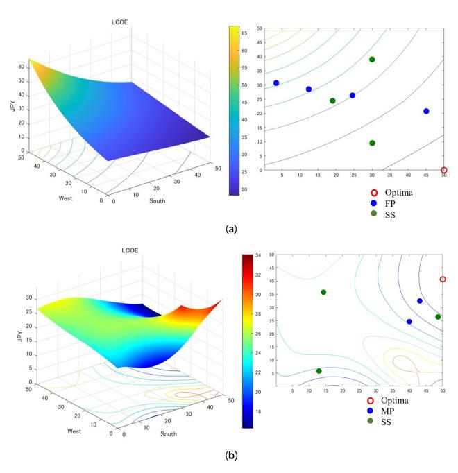
**Figure 14.** The SPV-GES LCOE variations (in the  $500 \times 500$  suburban simulation areas for (a) Fukuoka and (b) Ibaraki.
