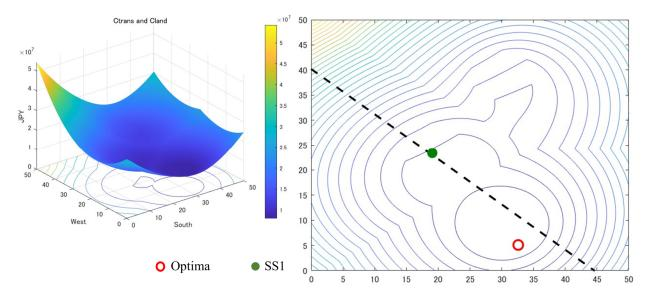
**Figure 15.** The location-dependent cost variations in the Fukuoka  $500 \times 500$  simulation area for SPV, based on transmission and land costs and SS1 only (dotted line represents the straight line connecting CBD and SS1 in Fukuoka).
