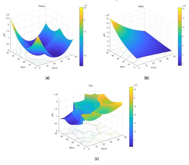
**Figure 10.** The SPV location-dependent cost variations in the  $500 \times 500$  Fukuoka suburban simulation area for (a) transmission ( $10^7$ ), (b) land ( $10^8$ ) and (c) supply chain ( $10^5$ ).
