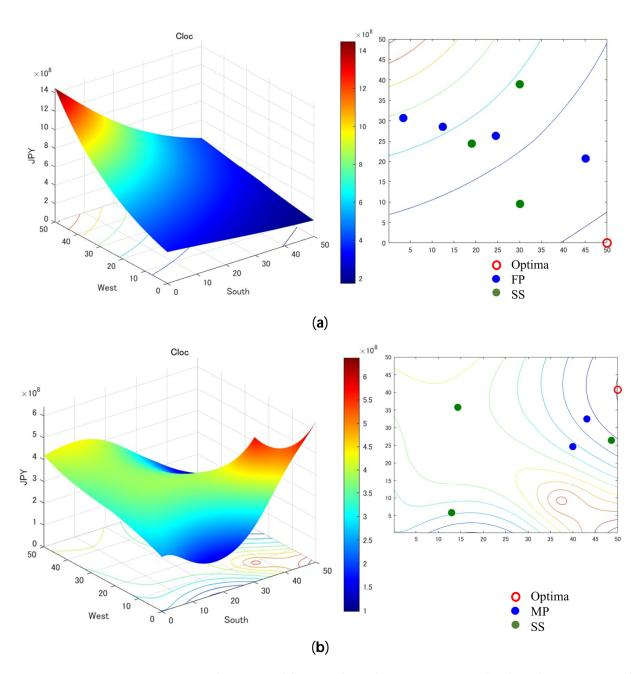
**Figure 12.** The SPV total location-dependent cost variations ( $C_{loc}$ ) in the 500  $\times$  500 suburban simulation areas for (**a**) Fukuoka (10<sup>8</sup>) and (**b**) Ibaraki (10<sup>8</sup>).
