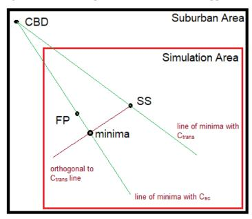
**Figure 16.** Geometrical approximation of the optimized cost location for a utility-scale GES installation in the suburban mountainous terrain of Fukuoka.
