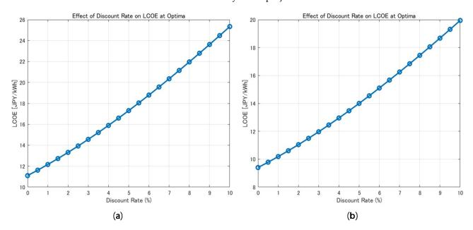
**Figure 20.** The variation of the LCOE at the cost-optimized locations in (a) Fukuoka and (b) Ibaraki simulation areas for the SPV-GES hybrid systems with discount rate (up to 10%).
