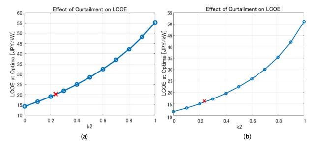
**Figure 18.** The variation of the LCOE at the cost-optimized locations in the (a) Fukuoka and (b) Ibaraki simulation areas for the SPV-GES hybrid systems with curtailment rate.
