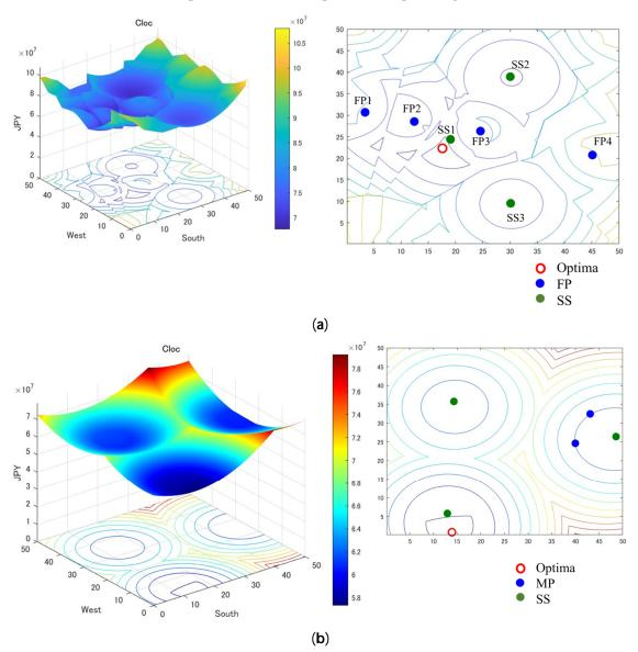
**Figure 8.** The GES total location-dependent cost variations ( $C_{loc}$ ) in the 500  $\times$  500 suburban simulation areas for (**a**) Fukuoka (10<sup>7</sup>) and (**b**) Ibaraki (10<sup>7</sup>).
