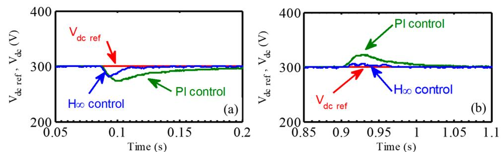
**Figure 10.** Experimental results of DC-link voltage under load disturbances comparison between conventional PI control and proposed  $H_\infty$  control: (a) load step change from 250  $\Omega$  to 110  $\Omega$  and (b) load step change from 110  $\Omega$  to 250  $\Omega$ .
