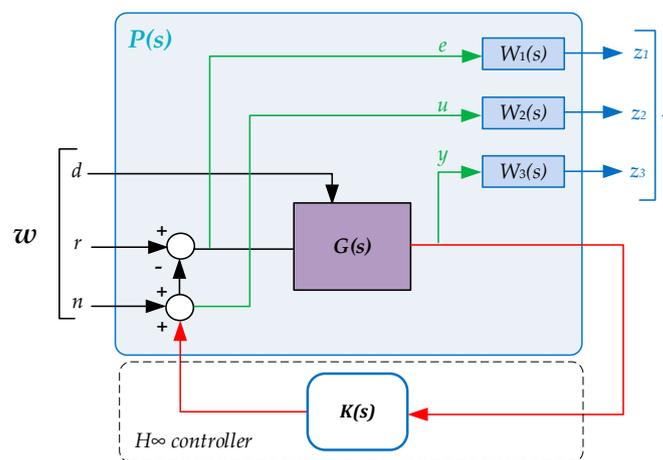
Figure 2. Weighted H-infinity control feedback structure.
