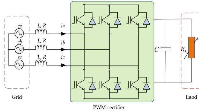
**Figure 1.** Grid-connected rectifier scheme.
