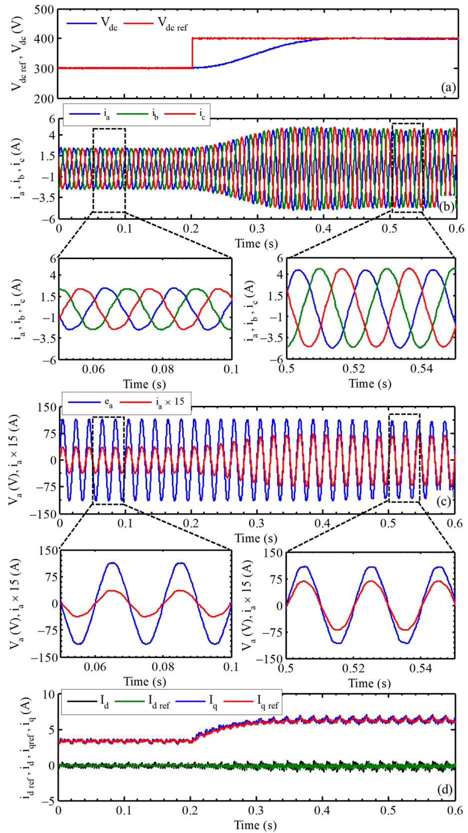
**Figure 7.** Experimental results under DC-link reference step change from 300 to 400 V: (a) DC-link voltages  $V_{dc}$  and  $V_{dc\ ref}$ ; (b) three-phase grid currents  $i_{abc}$ ; (c) grid current  $i_a$  and grid voltage  $e_a$  and (d)  $dq$ -axis current components and their references.
