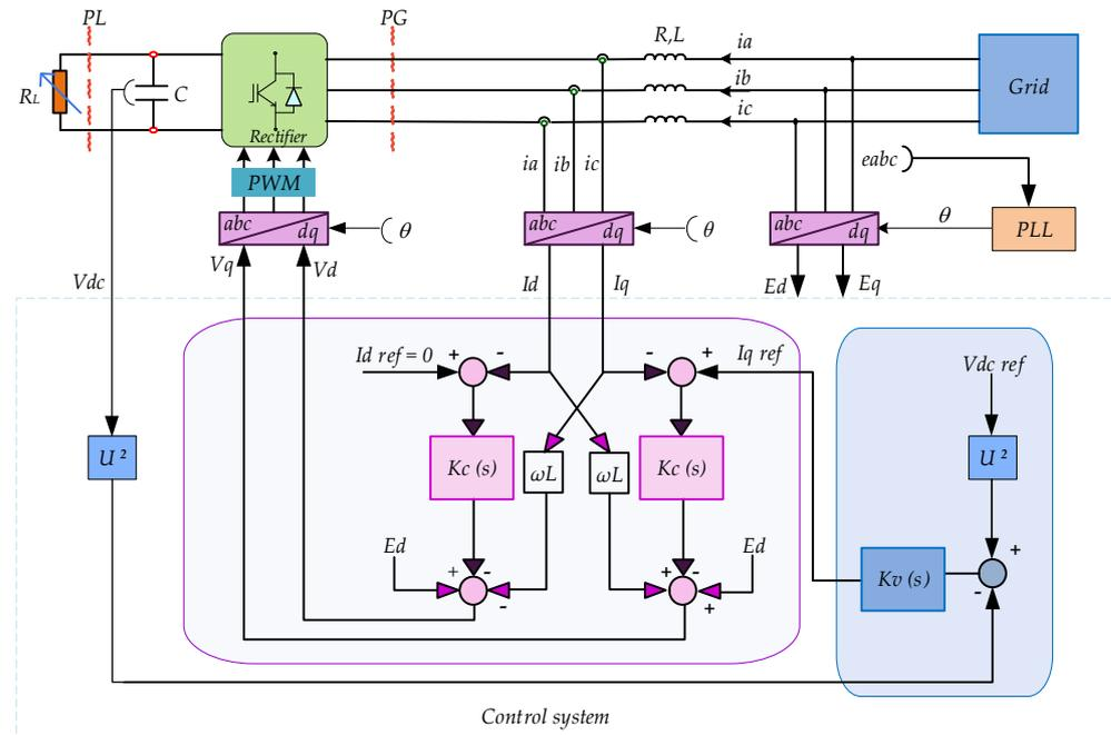
Figure 3. Proposed cascaded  $H_\infty$  control structure.
