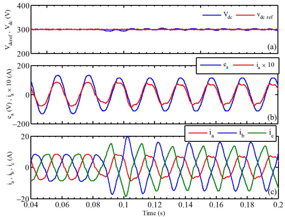
**Figure 9.** Experimental results under unbalanced grid voltage: (a) DC-link voltage  $V_{dc}$  and its reference  $V_{dc,ref}$ ; (b) grid current  $i_a$  and grid voltage  $e_a$  and (c) three-phase grid currents  $i_{abc}$ .
