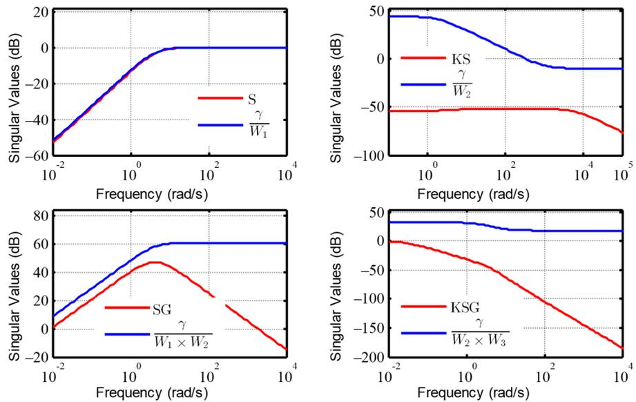
Figure 5. Graphical performances of closed outer loop responses and weighting functions.
