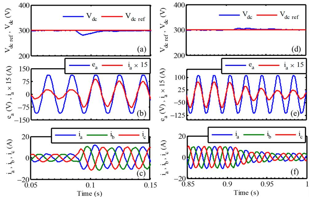
**Figure 8.** Experimental results under DC load disturbances: (a,d) DC-link voltage  $V_{dc}$  and reference  $V_{dc\ ref}$  waveforms; (b,e) grid current  $i_a$  and grid voltage  $e_a$  and (c,f) three-phase grid currents  $i_{abc}$ .
