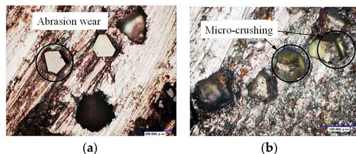
**Figure 2.** End face morphology of the diamond tool [19]: (a) common processing and (b) rotary ultrasonic processing.
