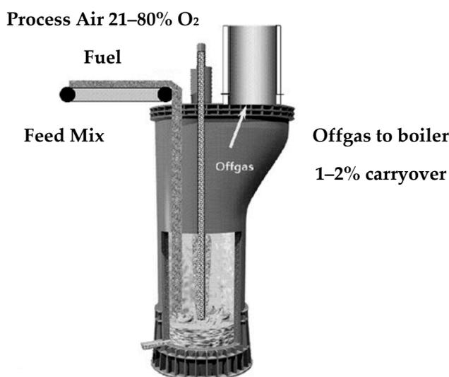
**Figure 4.** Scheme of Isasmelt technology [54].
