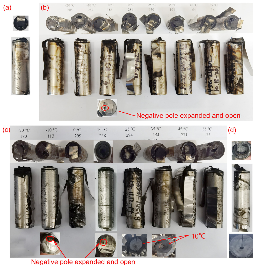
Figure 10. Pictures after thermal runaway. (a) Fresh battery; (b) 90% SOH; (c) 80% SOH; (d) failed battery.
