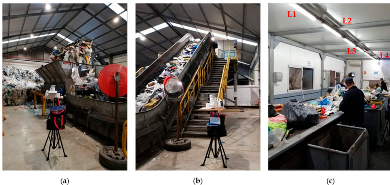
Figure 2. Photographs of WSU1: (a) unloading waste area and the feed hopper; (b) the ramp; (c) the cabin where the UV-C lamps are indicated as L1 to L4.
