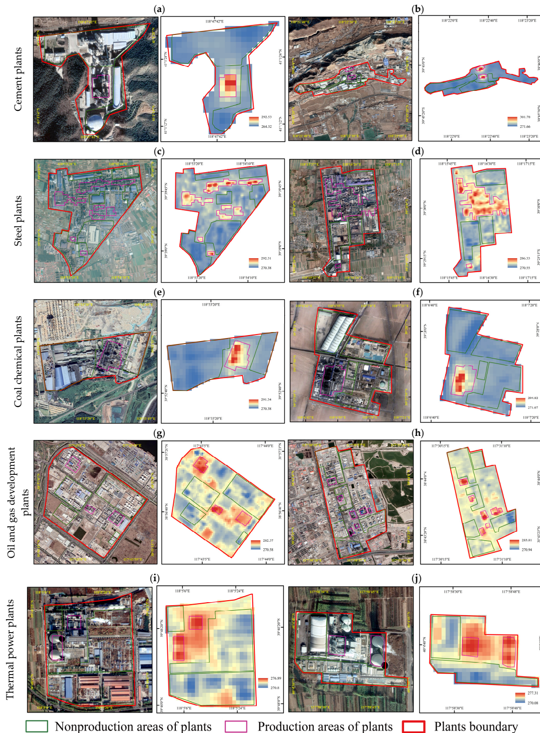
Figure 10. Google Earth images and satellite brightness temperatures based on SDGSAT-1 TIS Band 1 for different categories of industrial heat sources: (a) Jinyu Jidong Cement Pingquan Company
