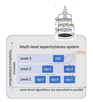
Figure 1. The sieve system is used to identify a CO in a 3DP job.
