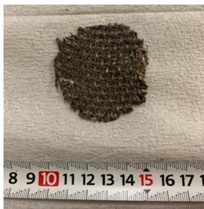
**Figure 13.** Photo of  $P_4O_{10}/TiO_2$  coated on the netlike glass disc.
