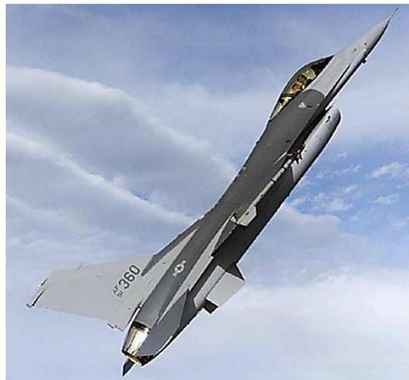
**Figure 35.** The F-16 features ventral fins positioned on the bottom of the fuselage, aft (rearward) of the wings. These ventral fins serve the purpose of stabilizing the aircraft during high-angle ascents and other maneuvers. However, the original design of the ventral fins experienced aerodynamic buffeting, resulting in a high failure rate [130].
