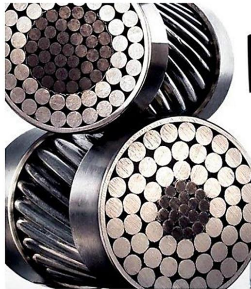
**Figure 36.** The cross-section of a 3M aluminum conductor composite-reinforced (ACCR) high-capacity MMC conductor used in overhead transmission lines consists of an aluminum core surrounded by Al-Zr outer wires. This design enhances strength, stiffness, and current-carrying capacity while minimizing weight and maximizing conductivity [11].
