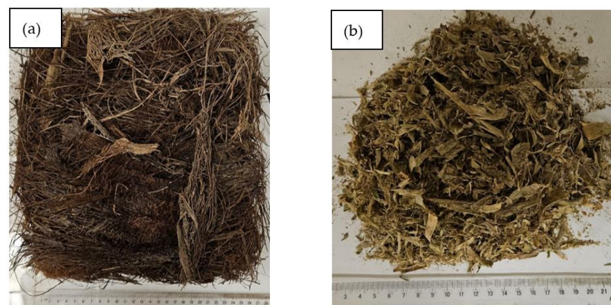
Figure 1. Loose fibers: (a) date palm surface fibers (DPSFs) and (b) pineapple leaf fibers.
