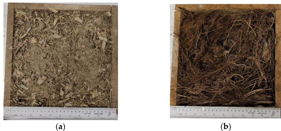
Figure 3. Loose fibers in the wooden mold: (a) PALF and (b) DPSF.
