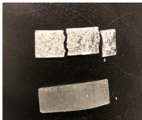
Figure 5. 3D printed resins LDO/AESO/TMPTA 18/66/16 wt% (0.5%wt of BAPO); top: without PAG; bottom: with 0.5%wt of PAG.
