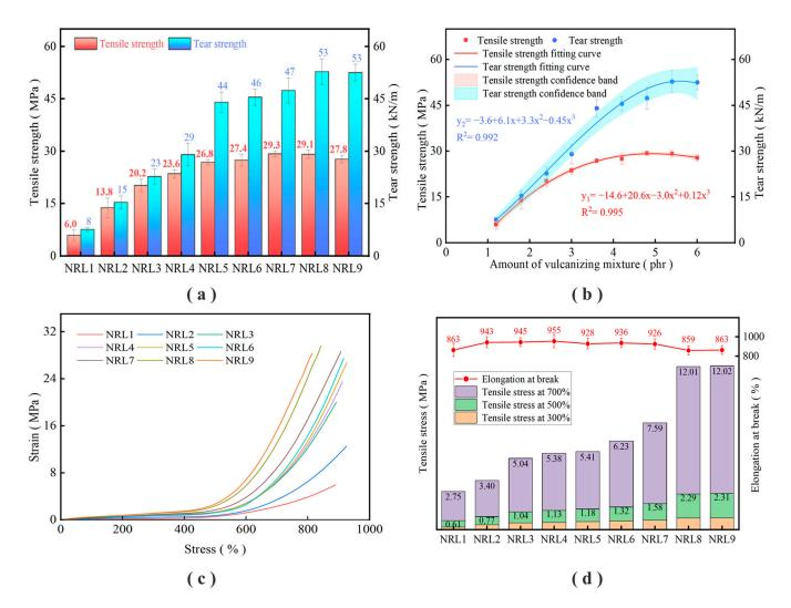
**Figure 2.** Mechanical properties of the film under different dosages of the vulcanization mixture: (a) mechanical properties of the film; (b) fitting curve of the mechanical properties; (c) stress–strain curve; (d) tensile stress and elongation at break.
