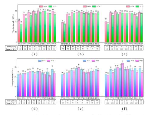
**Figure 6.** Test results of the mechanical properties of rubber film under different vulcanization conditions: (**a**–**c**) the tensile strength results of the film at 80 °C, 90 °C, and 100 °C, respectively; (**d**–**f**) the results of the tear strength of the film at 80 °C, 90 °C, and 100 °C, respectively.
