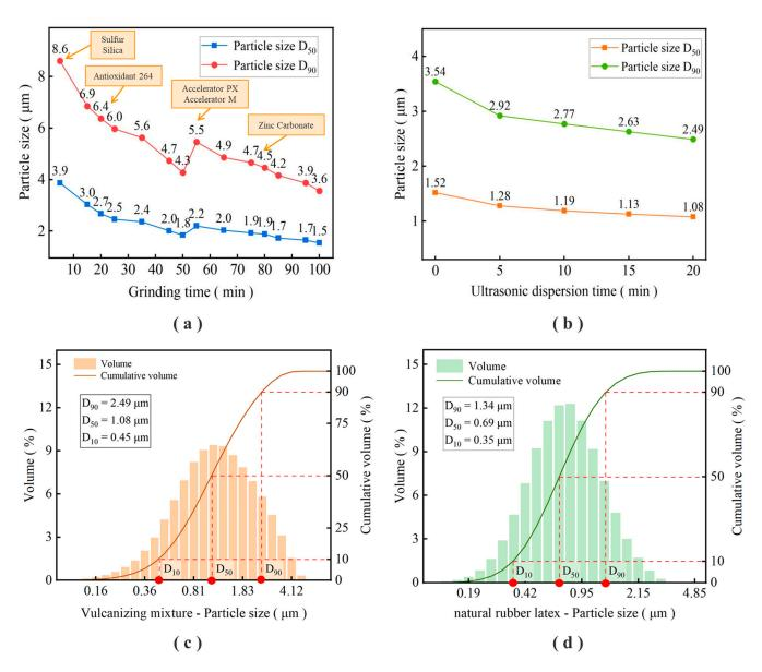
**Figure 1.** Refining process and particle size distribution curve of the vulcanized mixture: (**a**) particle size change during grinding of the vulcanization mixture; (**b**) particle size change during ultrasonic treatment of the vulcanization mixture; (**c**) particle size distribution of the final vulcanization mixture (**d**) particle size distribution of natural latex.
