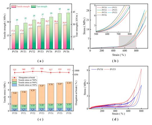
**Figure 5.** Test results of mechanical properties of the vulcanized film under different pre-vulcanization times: (**a**) tensile strength and tear strength; (**b**) stress–strain curve and local amplification diagram; (**c**) tensile strength and elongation at break; (**d**) cyclic tensile curve.
