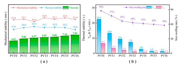
**Figure 4.** Properties of latex film under different pre-vulcanization times: (**a**) thermal stability, mechanical stability, and the viscosity of latex; (**b**) vulcanization characteristics and the dimensional swelling ratio of the film.
