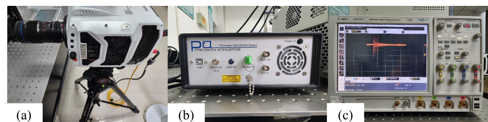
Figure 2. Signal collecting and testing equipment. (a) High-speed camera, (b) hydrophone, (c) oscilloscope.
