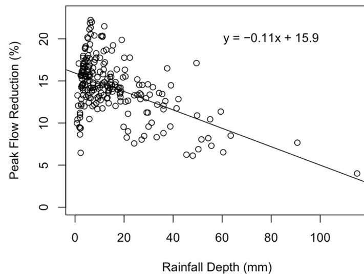
**Figure 5.** Relationship between peak flow reduction and rainfall depth for the 223 rainfall events, with linear regression line ( $p < 0.01$ ).
