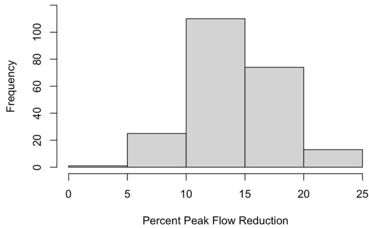
**Figure 4.** Histogram of percent peak flow reduction for the 100% rain garden implementation scenario (223 total events).
