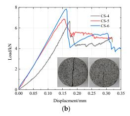
**Figure 3.** Brazilian splitting load-displacement curves of **(a)** rock-like material specimens and **(b)** sandstone specimens.
