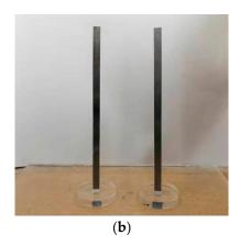
Figure 4. Prefabricated crack mould, (a) resin base, (b) steel sheet.
