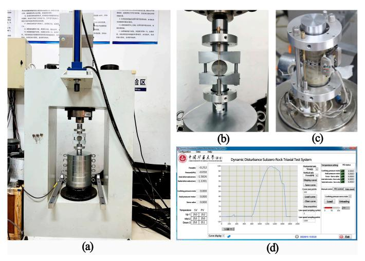
**Figure 1.** Test equipment, (a) loading system, (b) Brazilian splitting test, (c) uniaxial compression test, (d) software interface.
