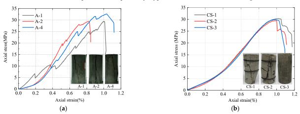
Figure 2. Stress-strain curves of (a) rock-like material specimens and (b) sandstone specimens.
