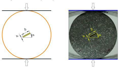
Figure 5. Schematic diagrams of size and flaw of disc specimen.
