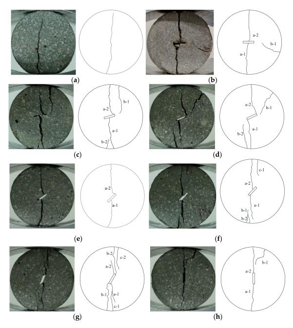
**Figure 9.** The ultimate failure mode of the intact specimen and pre-flawed specimens, (**a**) intact specimen, (**b**)  $\alpha = 0^{\circ}$ , (**c**)  $15^{\circ}$ , (**d**)  $30^{\circ}$ , (**e**)  $45^{\circ}$ , (**f**)  $60^{\circ}$ , (**g**)  $75^{\circ}$  and (**h**)  $90^{\circ}$ .
