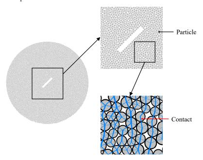
Figure 14. Typical numerical model specimen.
