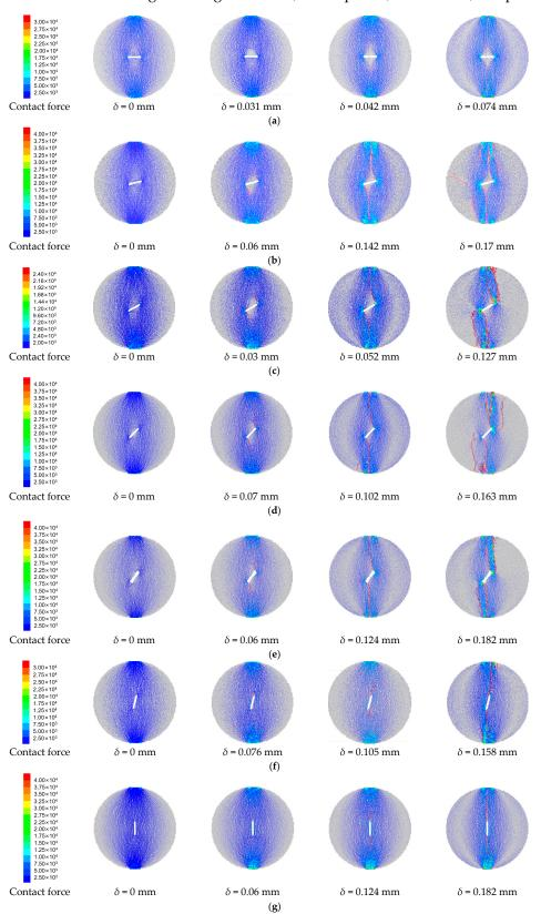
**Figure 15.** The evolution laws of contact force and crack, (**a**)  $\alpha = 0^{\circ}$ , (**b**)  $15^{\circ}$ , (**c**)  $30^{\circ}$ , (**d**)  $45^{\circ}$ , (**e**)  $60^{\circ}$ , (**f**)  $75^{\circ}$  and (**g**)  $90^{\circ}$ .
