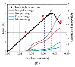
**Figure 19.** Energy evolution curve of single-flawed model, (**a**) main energy evolution, (**b**) dissipation energy evolution, (**c**) elastic strain energy evolution.
