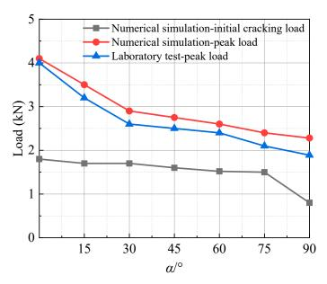
Figure 18. Relationship between peak load and flaw dip angle.
