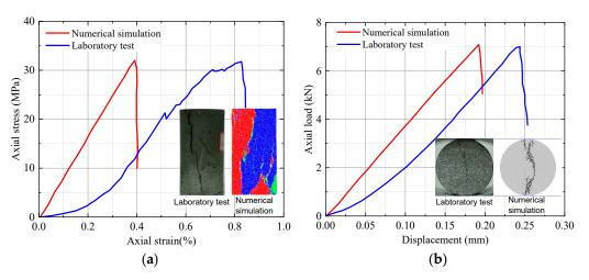
Figure 13. Comparison of test and simulation results, (a) uniaxial compression test, (b) Brazilian Split test.
