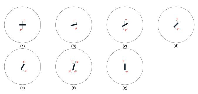
**Figure 10.** Crack propagation type in Brazilian disc with a single flaw, (**a**)  $\alpha = 0^{\circ}$ , (**b**)  $15^{\circ}$ , (**c**)  $30^{\circ}$ , (**d**)  $45^{\circ}$ , (**e**)  $60^{\circ}$ , (**f**)  $75^{\circ}$  and (**g**)  $90^{\circ}$ .
