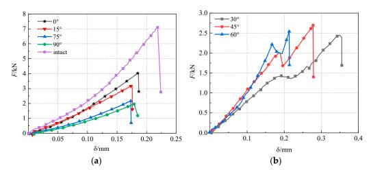
Figure 6. Load-displacement curves of disc specimens under Brazilian test, (a) type I, (b) type II.
