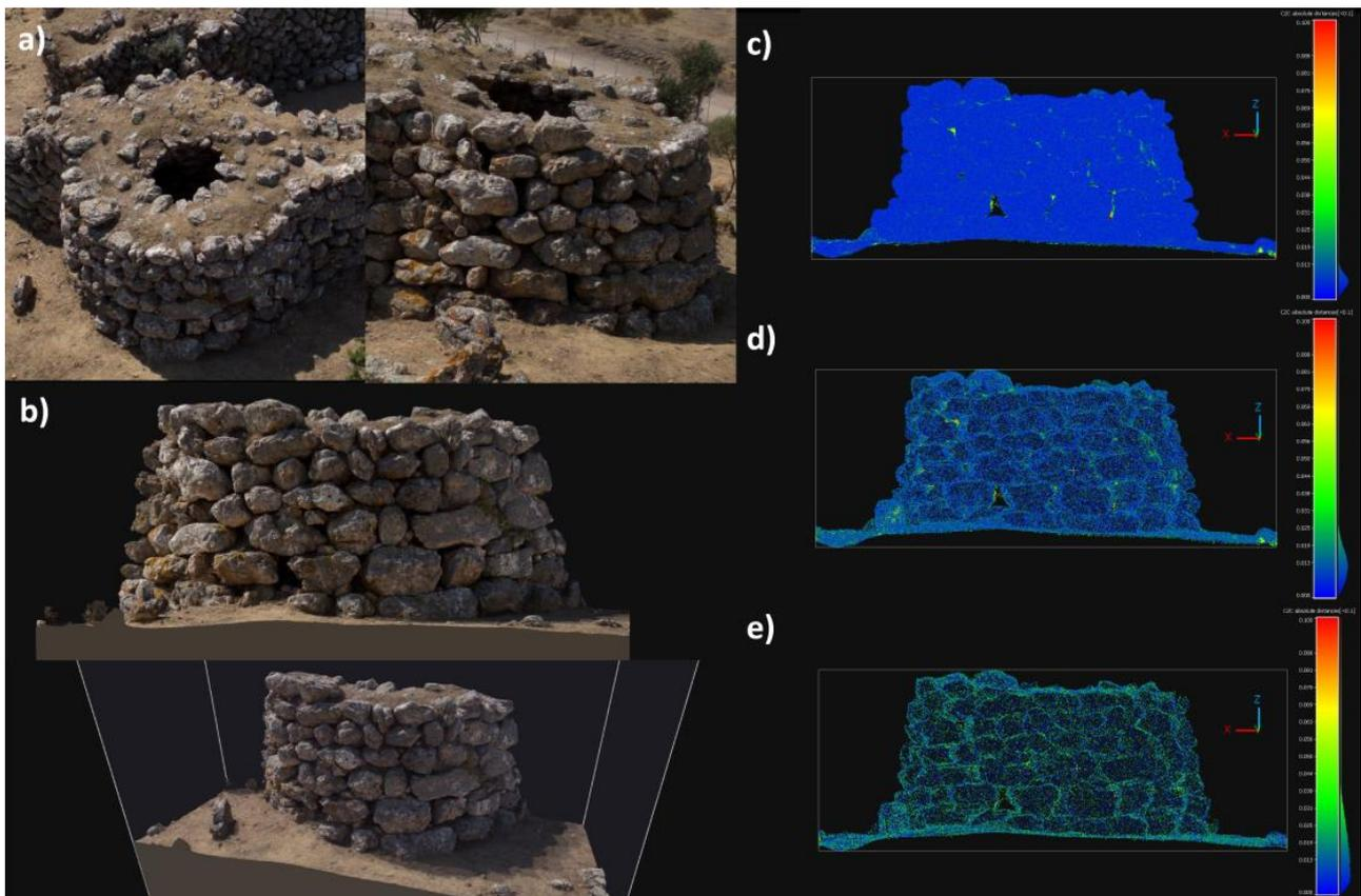
**Figure 15.** (a) Top view from north of detail tower M; (b) example of model surface for C2C comparison: the wall of tower M, with the 3D model delimited by the reconstruction region (RR<sub>4</sub>); (c) the calculated distance from C2C of point clouds M1 and M2; (d,e) the calculated C2C error distance from point clouds with progressive simplification of the minimal edge length.
