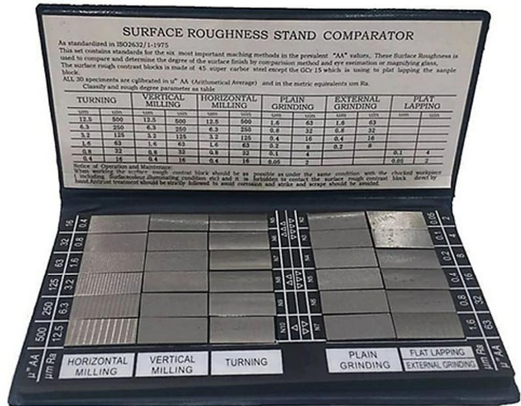
Figure 11. Surface roughness comparator standards composite set.
