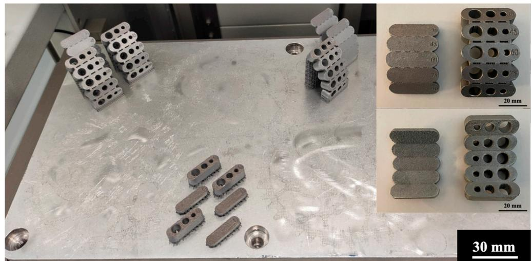
**Figure 4.** L-PBF-produced structures on the build platform. The figure presents also some insets showing the surface quality of the produced parts.
