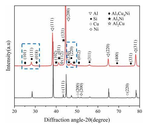
Figure 1. XRD of powder and as-built sample of Al-Si-Cu-Ni.
