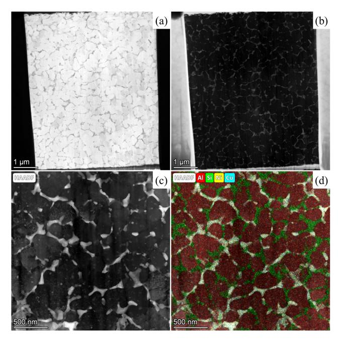
**Figure 3.** TEM images of microstructural characteristics on the top surface of PBF-LB/M Al-Si-Cu-Ni samples: (**a**) bright-field image; (**b**) dark-field image; (**c**) HAADF morphology; (**d**) EDS mapping element distribution.
