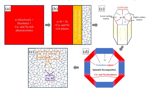
**Figure 5.** Schematic diagram of the formation of the cellular structure of PBF-LB/M Al-Si-Cu-Ni: (a) melt, (b–c) flow of high melting point phases, (d) spinodal decomposition and (e) cellular structure.
