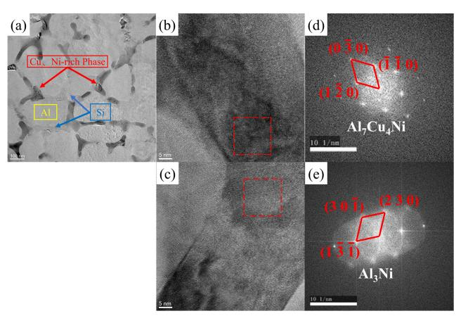
**Figure 4.** TEM images of PBF-LB/M Al-Si-Cu-Ni samples: (a) bright-field image of  $\alpha$ -matrix and cellular structure; (**b**–**e**) HRTEM images of Al<sub>7</sub>Cu<sub>4</sub>Ni, Al<sub>3</sub>Ni, and FFT results of the corresponding regions.
