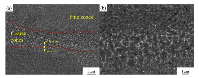
**Figure 2.** The microstructure of Al-Si-Cu-Ni samples: (**a**) low magnification; (**b**) enlarged view of the yellow box in (**a**).
