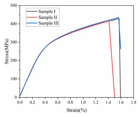
Figure 7. Tensile property of PBF-LB/M Al-Si-Cu-Ni alloy.
