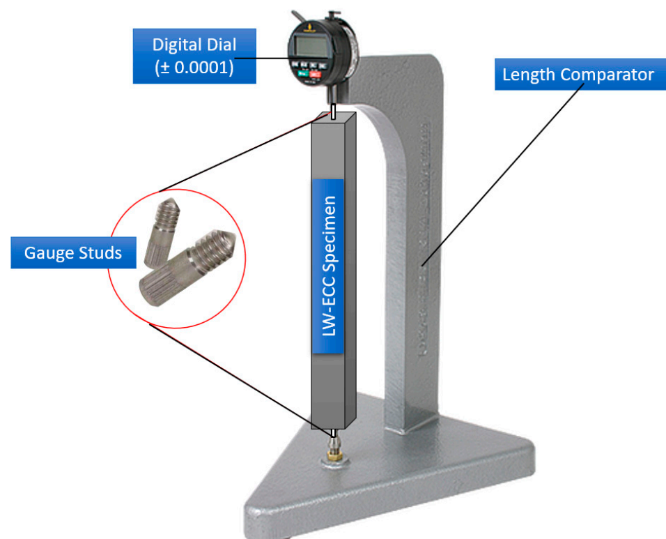
Figure 2. Shrinkage Test Set up.
