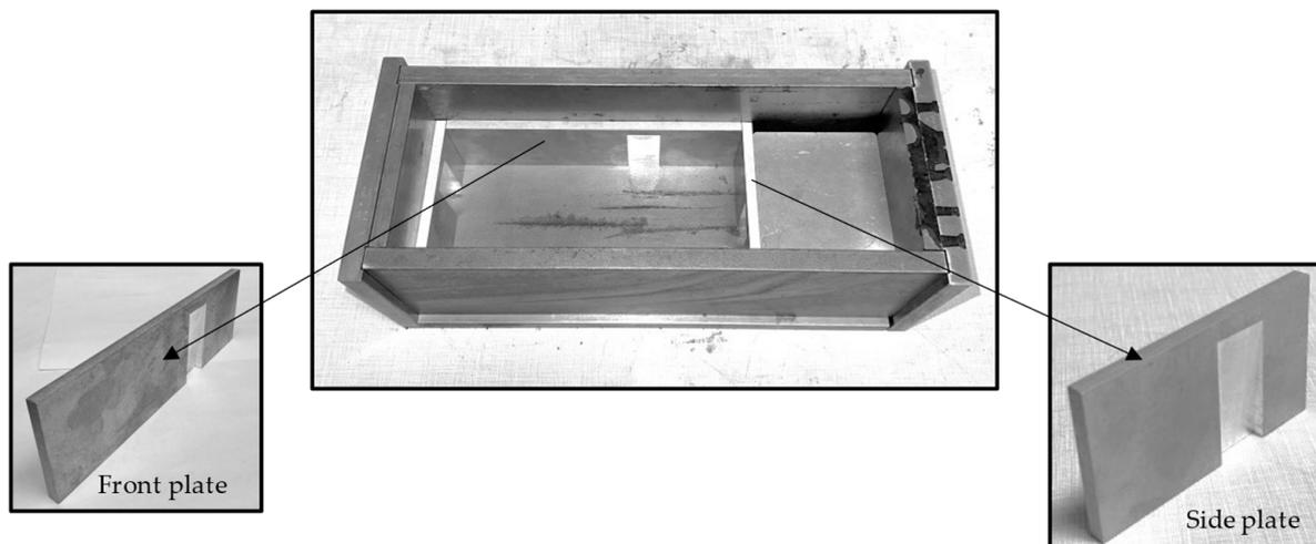
**Figure 2.** High-strength steel mold and specifically designed front and side plates made of aluminum for giving protrusions to the char-based paving blocks.
