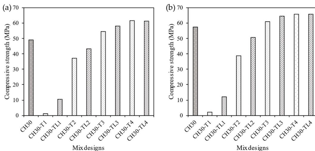
**Figure 10.** Comparison of compressive strength of char-based paving blocks based on various mix designs: (a) 7-day test results and (b) 28-day test results.
