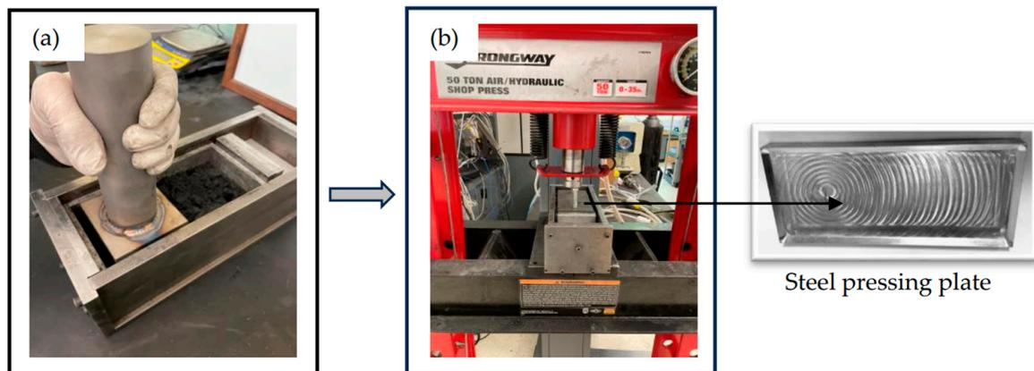
**Figure 3.** Stages in developing process of char-based paving block: (a) initial compaction with cylindrical hammer and (b) final compression using a hydraulic press.
