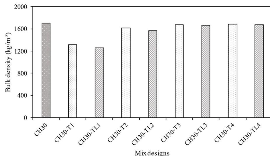
**Figure 9.** Comparison of bulk density of char-based paving blocks based on various mix designs.
