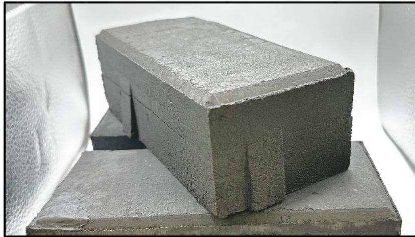
**Figure 4.** Char-based paving block with protrusions.
