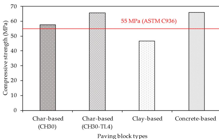
**Figure 11.** Comparison of compressive strength of char-based paving blocks with clay- [41] and concrete- [23] based paving blocks.
