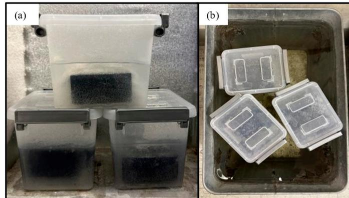
**Figure 8.** Half-sized block samples in the (a) freezing chamber and (b) thawing tank.
