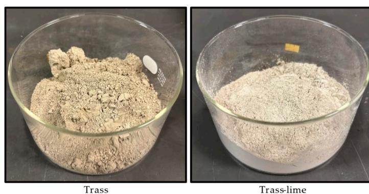
**Figure 1.** Pozzolanic materials (trass and trass-lime) used for manufacturing char-based paving blocks.
