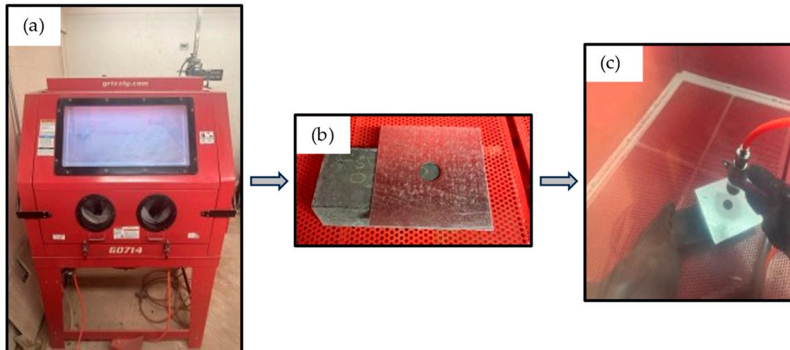
**Figure 6.** Determination of abrasive resistance of paving blocks: (a) sand abrasion equipment used in the study, (b) arrangement of sample setup inside the equipment, and (c) injection of abrasive materials over the sample.
