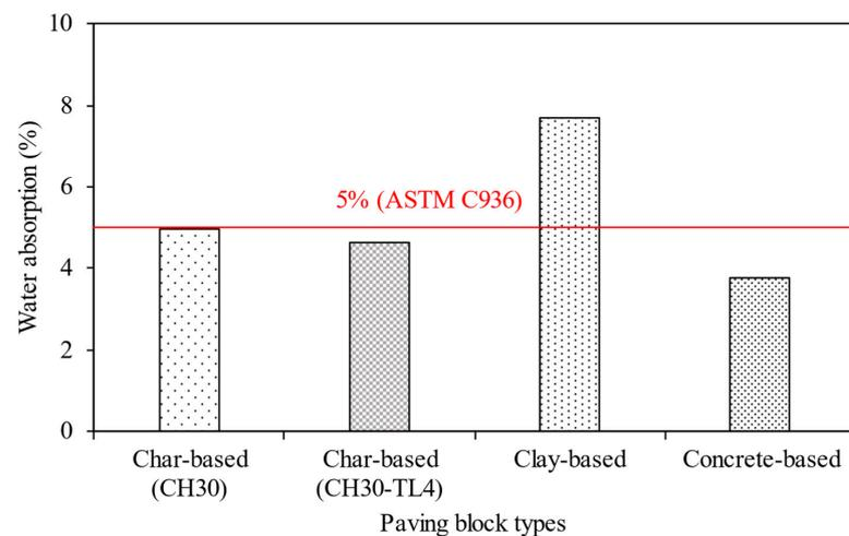
**Figure 13.** Comparison of water absorption of char-based paving blocks with clay- [41] and concrete- [51] based paving blocks.
