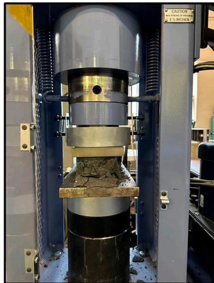
**Figure 5.** Measurement of compressive strength of char-based paving blocks.
