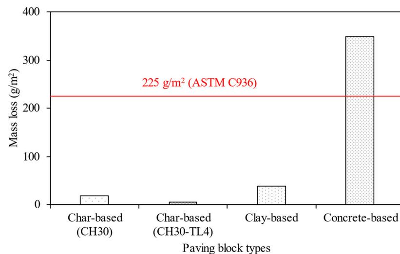
**Figure 14.** Comparison of freeze–thaw test results of char-based paving blocks with clay- [41] and concrete- [54] based paving blocks.
