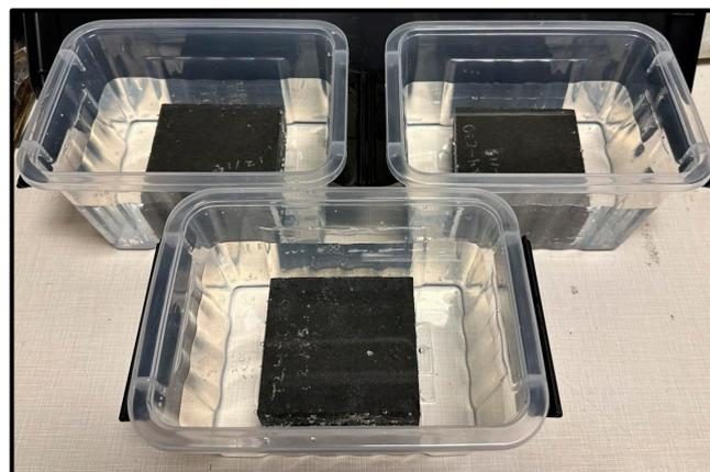
**Figure 7.** Half-sized block samples submerged in water for water absorption test.
