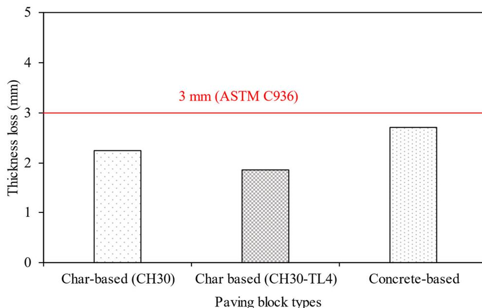
**Figure 12.** Comparison of abrasion resistance of char-based paving blocks with concrete-based [49] paving blocks.
