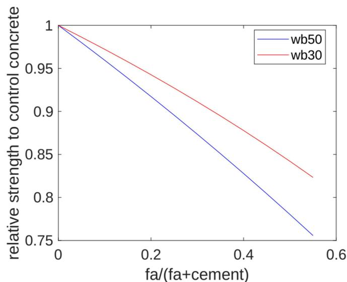
**Figure 3.** Effects of water/binder ratio and fly ash/binder ratio on relative strength of material.
