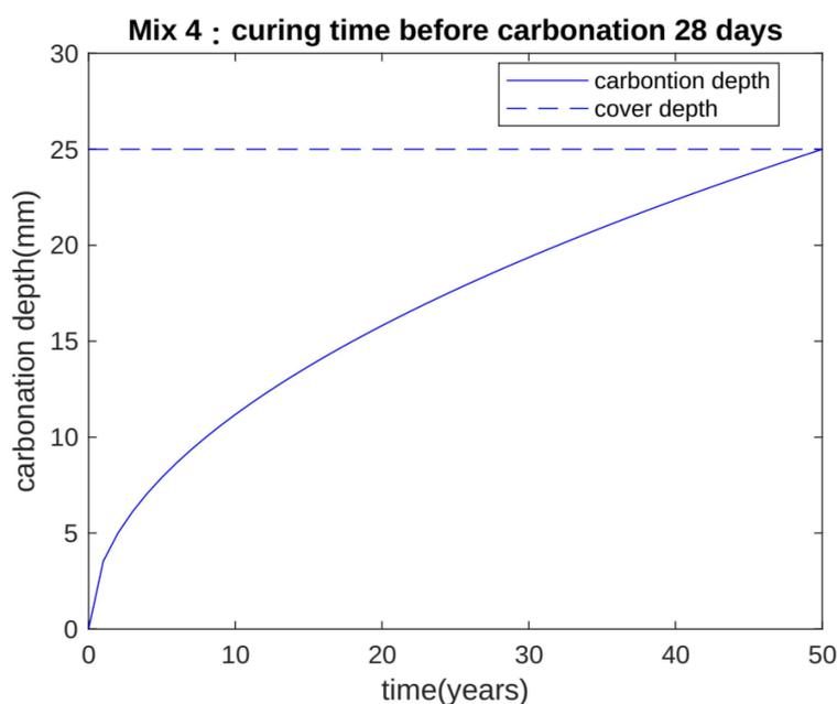
Figure 9. Carbonation depth curve of Mix 4.
