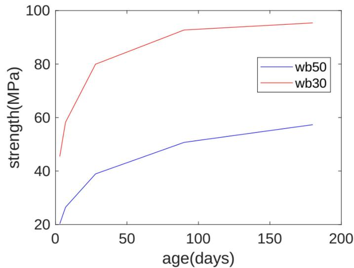
**Figure 4.** Effects of water/binder ratio and age on strength.
