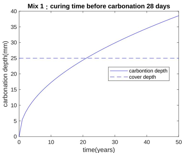
**Figure 6.** Carbonation depth curve of Mix 1.
