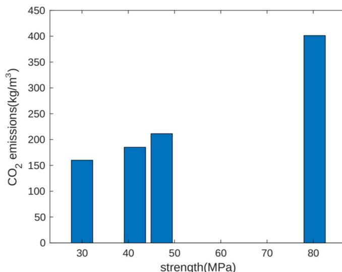
**Figure 10.** The relationship between strength and carbon emissions.
