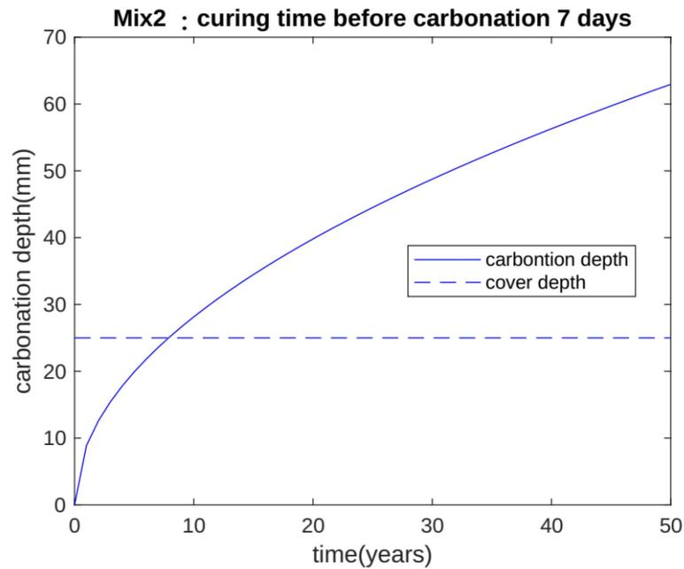
Figure 7. Carbonation depth curve of Mix 2.
