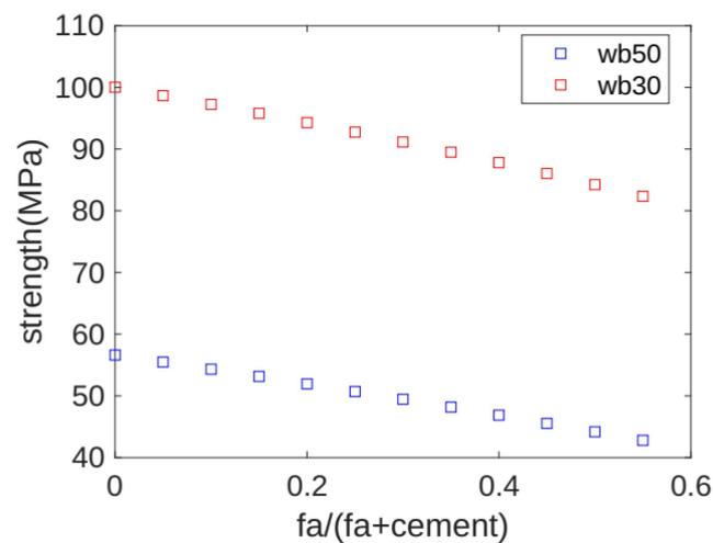
**Figure 2.** Effects of water/binder ratio and fly ash/binder ratio on strength.
