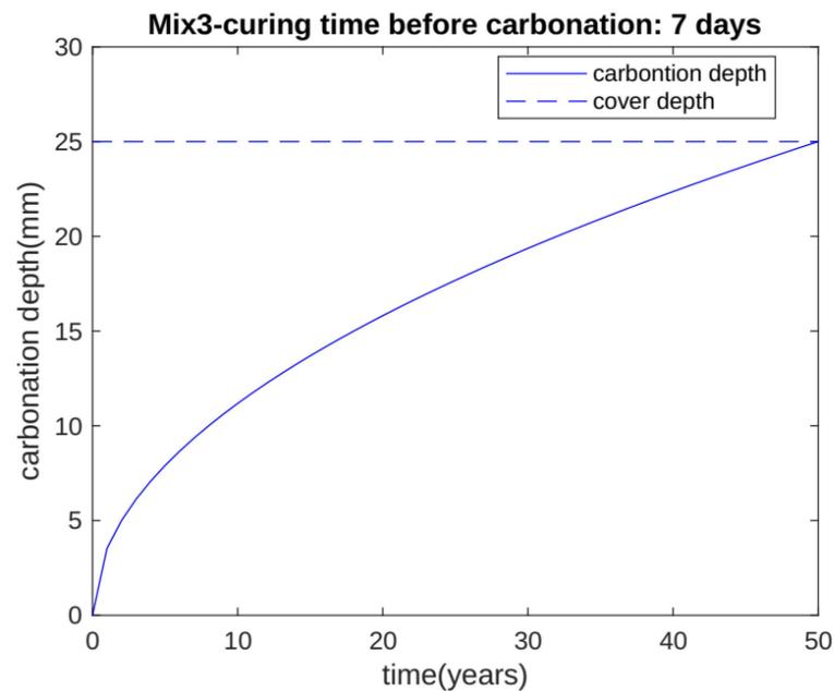
Figure 8. Carbonation depth curve of Mix 3.
