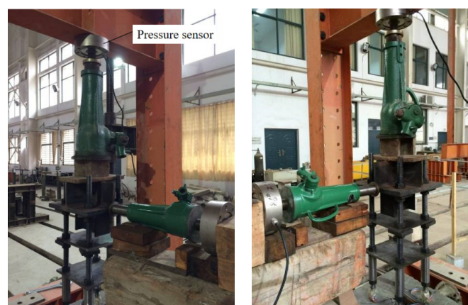
Figure 14. Diagram of load application.
