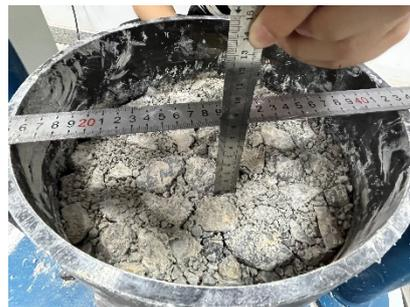
**Figure 2.** The measurement of the specimen height.
