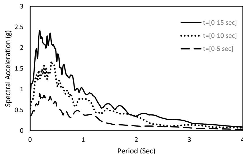
**Figure 6.** Spectral acceleration of the endurance time function at different time ranges.
