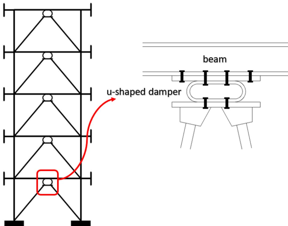
**Figure 1.** Schematic installation view of U-shaped damper.
