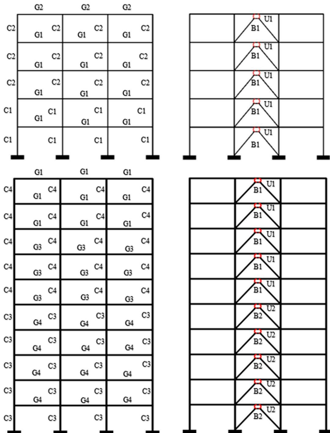
**Figure 3.** Schematic view of the studied original and retrofitted structures.
