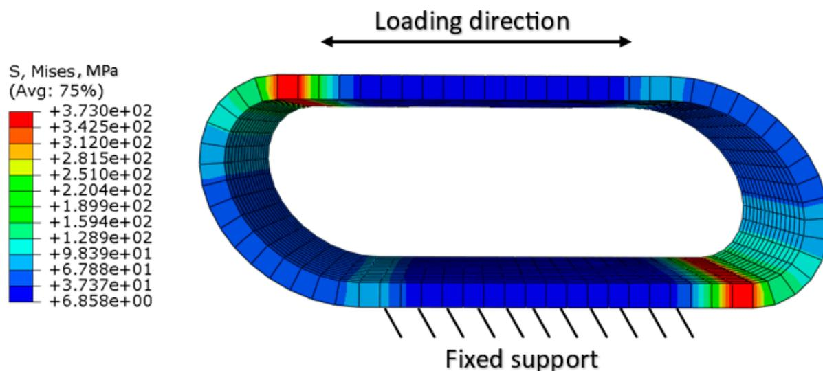
**Figure 2.** Developed stresses on a U-shaped damper.
