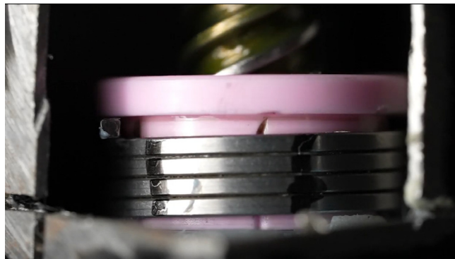
Figure 16. High-speed camera images captured of the improved overrunning spring clutch.
