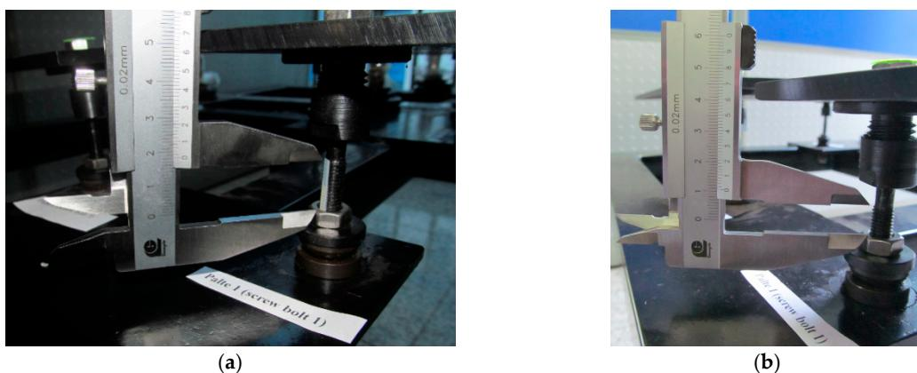
**Figure 11.** The support distance of bolt 1 before and after alignment in Plate 1 using the three-rotation alignment method: (a) before alignment, distance is 18.40 mm and (b) after alignment, distance is 10.82 mm.
