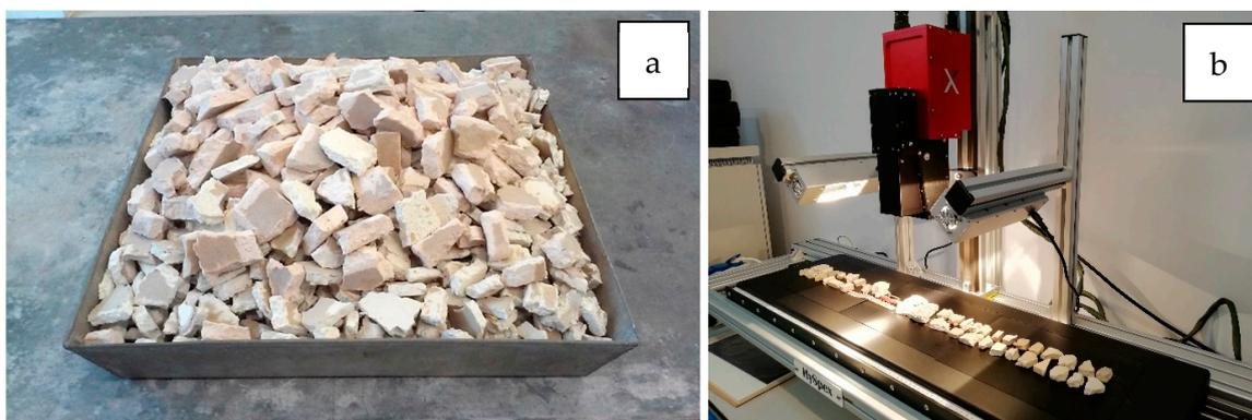
**Figure 2.** Refurbishment plasterboard waste fragments composed of gypsum core and lining paper (a) and laboratory-scale experimental setup with advanced HSI camera, air-cooled tubular halogen lamps and sliding scanning table for in-line material classification (b).
