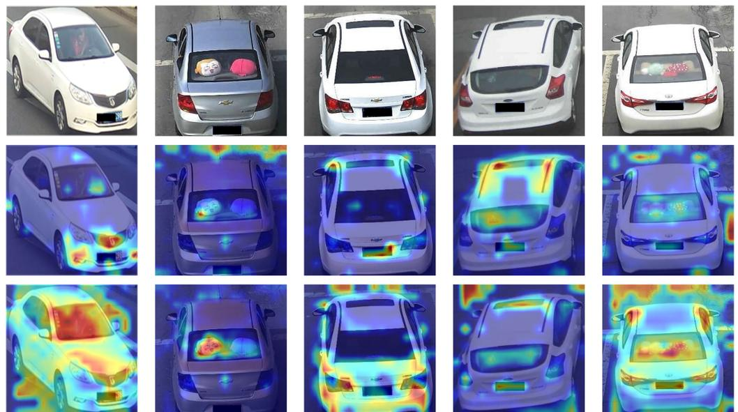
Figure 4. The Grad-CAM visualization of attention maps. The first, second, and third rows show the original image, Baseline, and SaGT, respectively.
