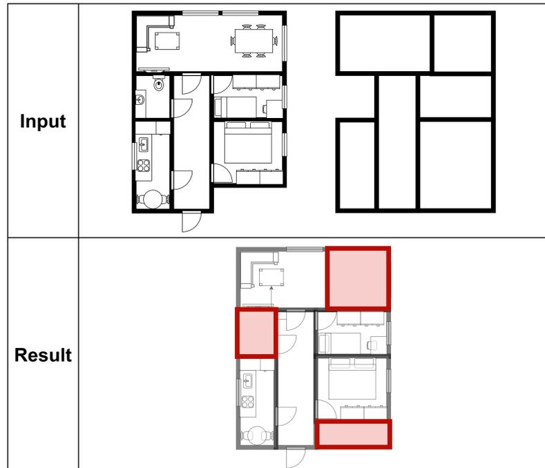
**Figure 12.** Visualization of the Change Detection task. Initial and updated images (**top**) are analyzed and searched for differences between them. Detected mismatched elements are marked in red (**bottom**).
