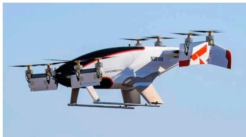
**Figure 1.** Test evtol for Airbus A3: Vahana.
