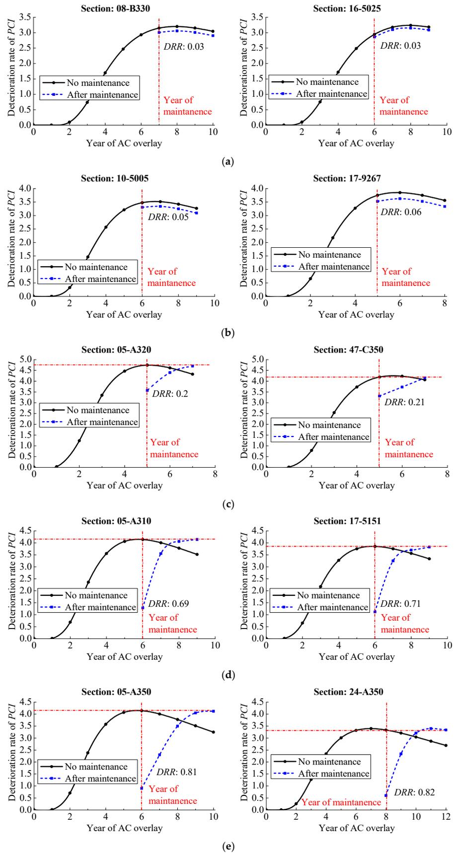
**Figure 6.** Deterioration rate of PCI versus year of AC overlay of sections treated with various preventive maintenance technologies. (a) Crack sealing; (b) Crack filling; (c) Fog seal; (d) Thin HMA overlay; (e) Hot-mix recycled AC.
