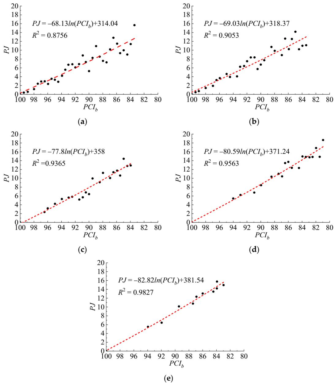
**Figure 5.**  $PJ$  versus  $PCI_b$  of sections treated with five different preventive maintenance technologies. (a) Crack sealing; (b) Crack filling; (c) Fog seal; (d) Thin HMA overlay; (e) Hot-mix recycled AC.
