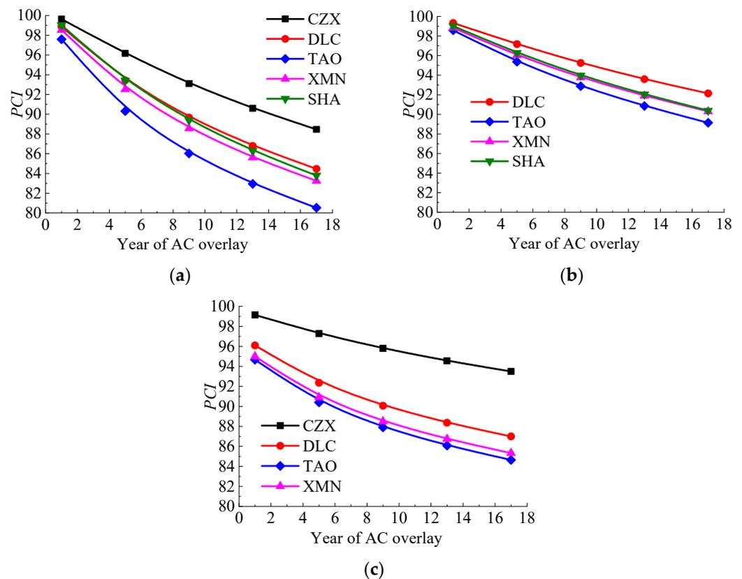
Figure 4. PCI deterioration curves of different composite pavement regions. (a) Middle runway; (b) Terminal runway; (c) Taxiway.
