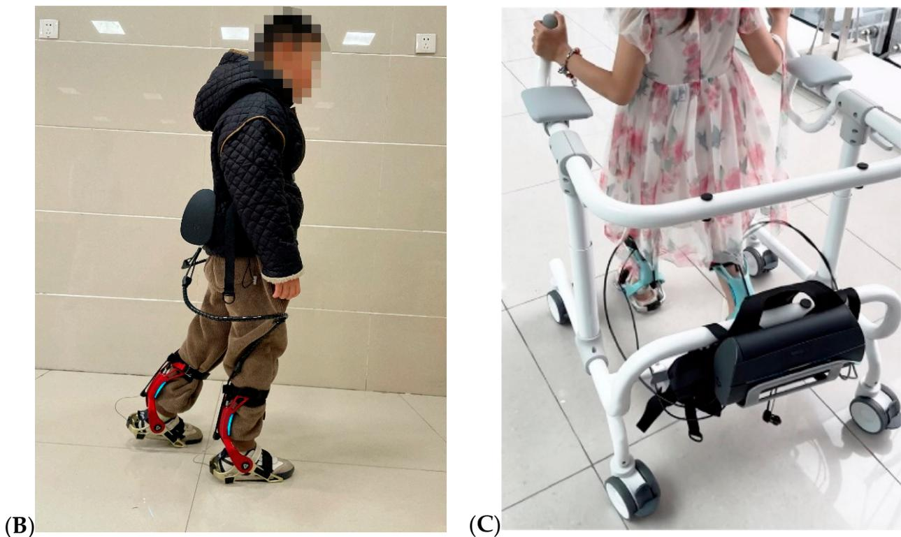
**Figure 2.** (A) Relink-ANK soft robotic exoskeleton, (B) SRE-assisted overground walking training, (C) SRE-assisted overground walking training with a walking aid.
