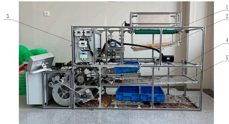
**Figure 17.** Test rig for screen load homogenization of discharged material for threshing in longitudinal axial flow. (1). Feed box. (2). Return plate. (3). Electronic control system. (4). Cleaning sieve. (5). Receiving box.
