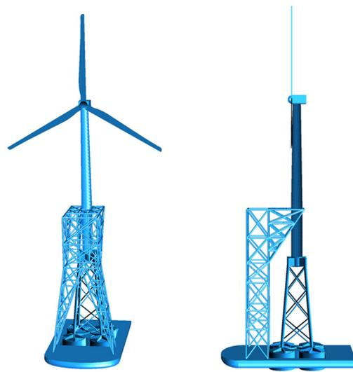
**Figure 4.** Integrated transportation concept of the FBJF.
