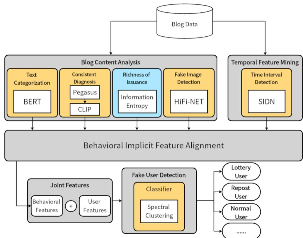
Figure 1. Network architecture of MAPM.
