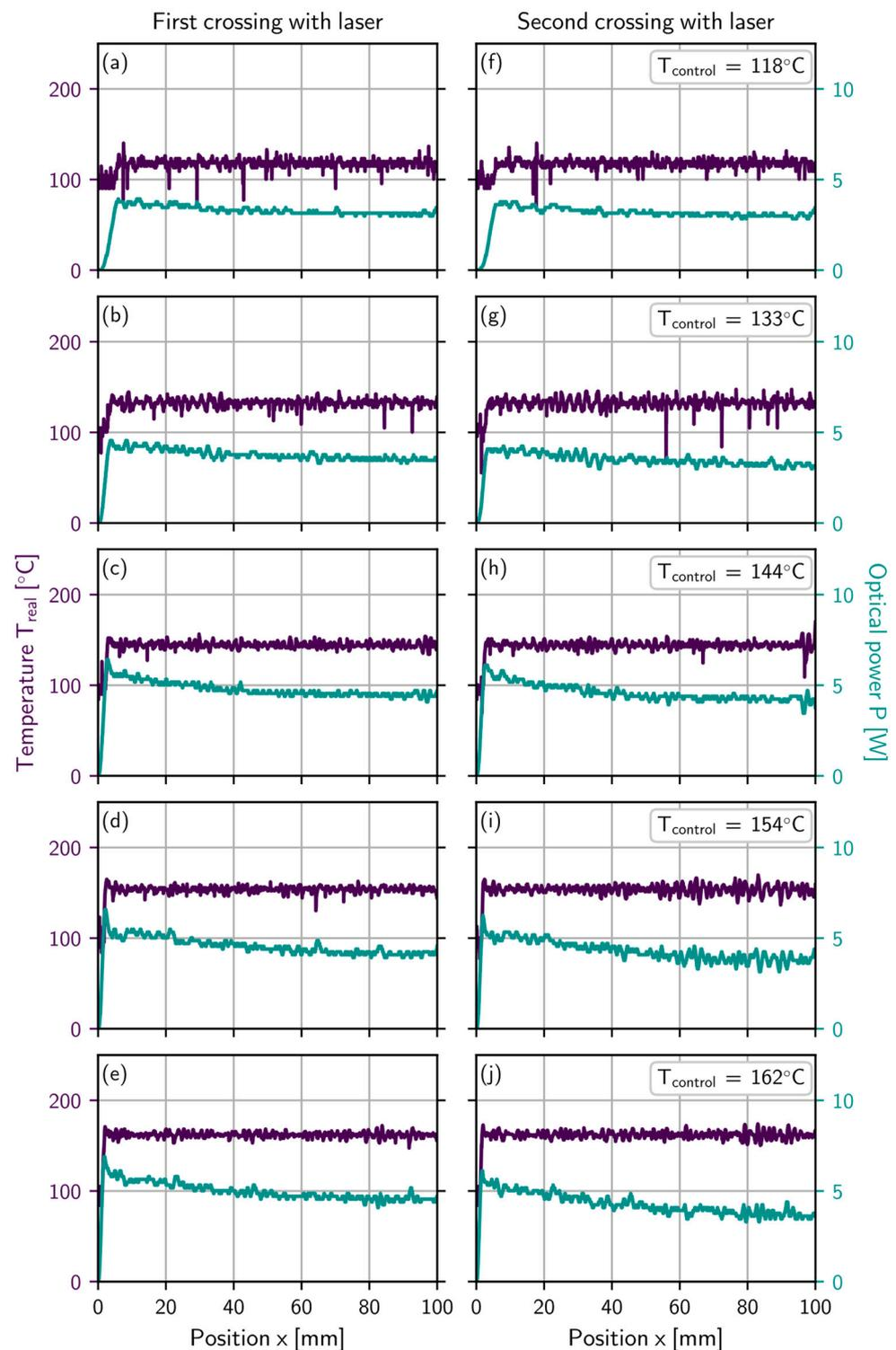
**Figure 7.** Measurement of the temperature and optical power of the laser during first (a–e) and second (f–j) crossing with the laser over the conductive tracks for different control temperatures at every position.
