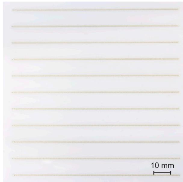
**Figure 2.** Photography of samples used: polycarbonate substrate with 11 printed conductive lines produced from silver paste 1901-SB. Length of each line is 100 mm, width of each line is approximately 0.75 mm, cross-section before curing is approximately 0.055 mm.
