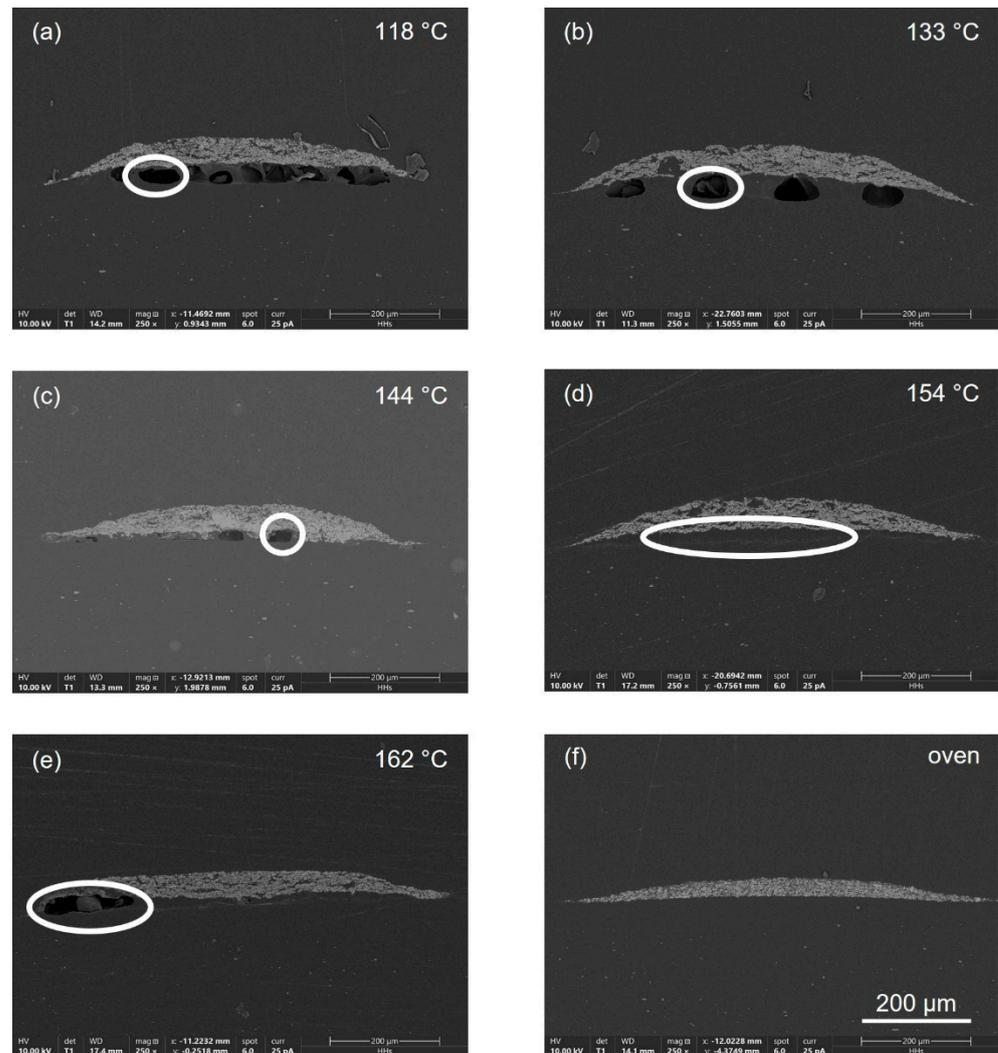
**Figure 12.** SEM images of cross-section polishes of the fabricated traces: laser-processed with a set temperature of (a) 118 °C, (b) 133 °C, (c) 144 °C, (d) 154 °C, (e) 162 °C; (f) oven-processed. Air inclusions due to laser processing are shown in white.
