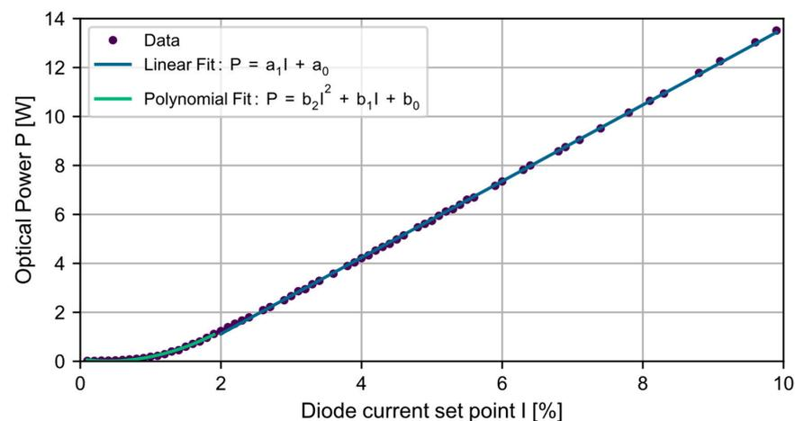
**Figure 5.** Measurement and fitted model for the correlation between the diode current set by the pyrometer and the optical power measured. Due to the non-linear behavior of the optical power for a diode current set point under 2%, a quadratic correlation is assumed here.
