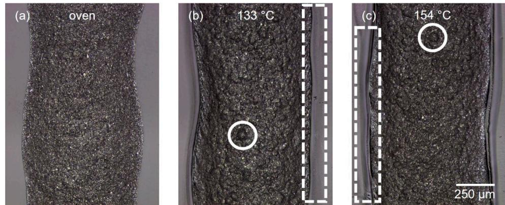
**Figure 11.** Comparison of the pictures recorded by LSM: (a) oven-processed, (b) laser-processed with a set temperature of 133 °C, (c) laser-processed with a set temperature of 154 °C. The white circles mark gas bubbles that were generated in the layer and did not escape; the white dashed rectangles show condensed residues of the solvents on the substrate surface.
