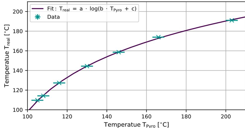
**Figure 6.** Calibration curve of the pyrometer for converting the measured temperatures into the temperature at the coating surface. A function of type  $T_{real} = a \log(b T_{Pyro} + c)$  is used to fit the data.
