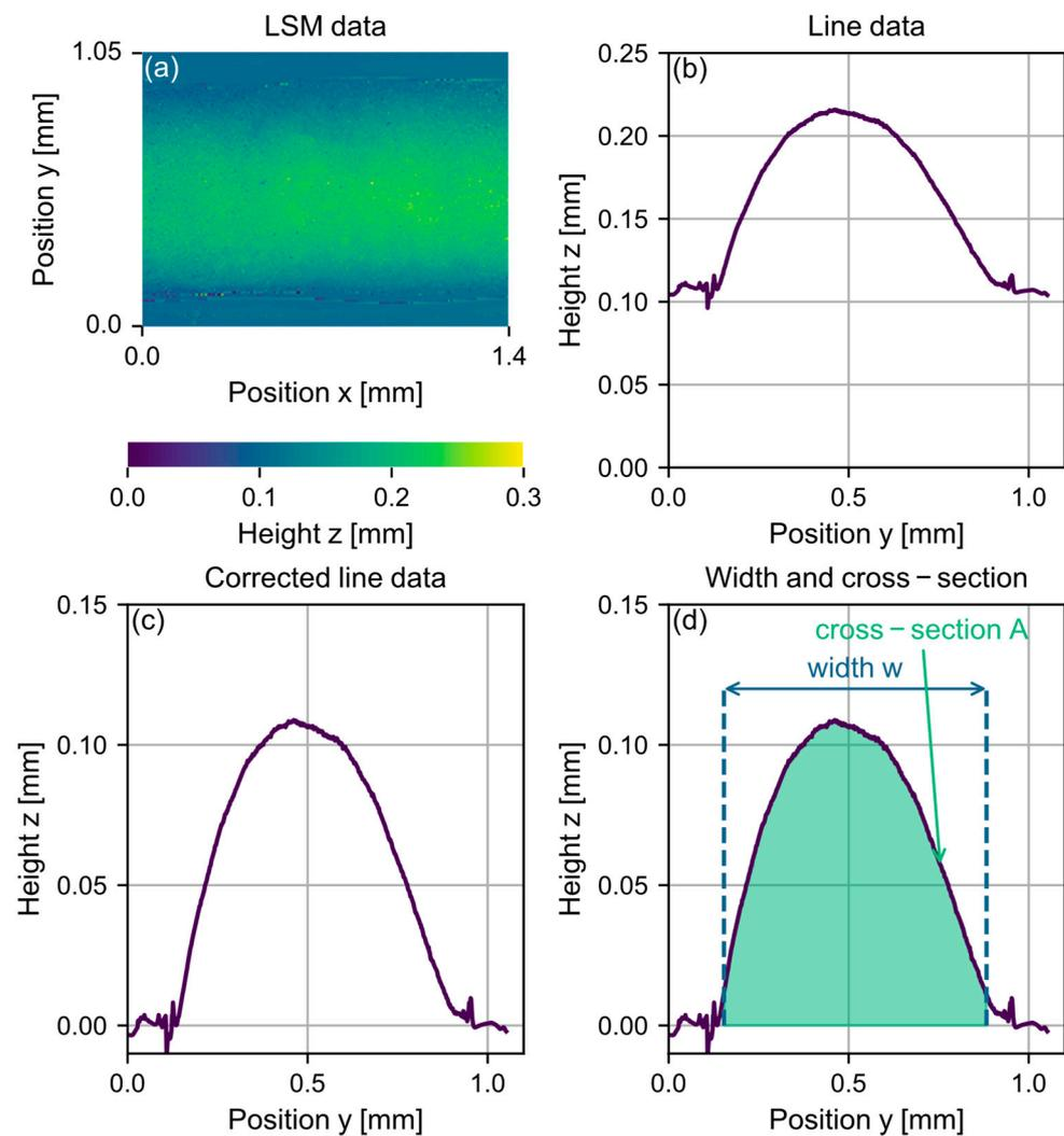
**Figure 9.** Method used for the analysis of the geometric properties of the cured traces: the height information from an LSM measurement (a) is averaged in terms of the direction  $x$  (b), and then corrected by linear regression (c). The width  $w$  or the cross-section  $A$  is determined by the difference or the integral between the first and the last points with a value of at least  $0.1 z_{\max}$  (d).
