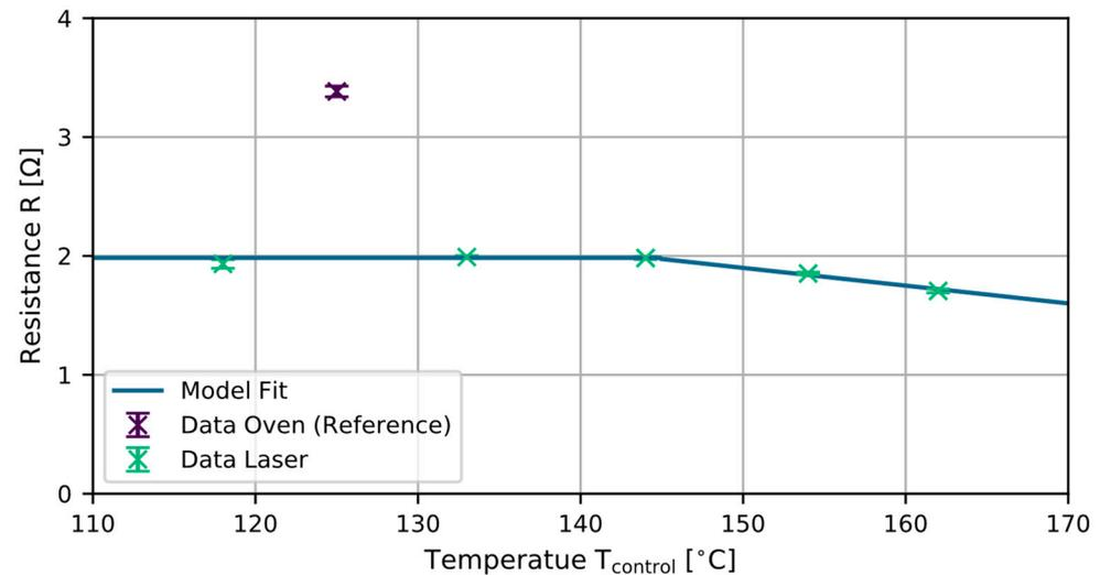
**Figure 8.** Resulting electrical (ohmic) resistance of the traces as a function of the set control temperature. A constant and a linear function is used to describe the resistance as a function of the temperature.
