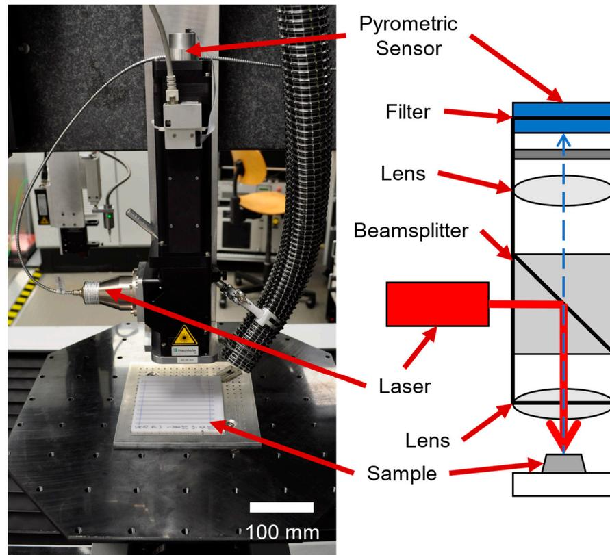
**Figure 4.** (Left): photography of the experimental setup used. (Right): schematic representation of the optical setup for laser beam as well as pyrometry.
