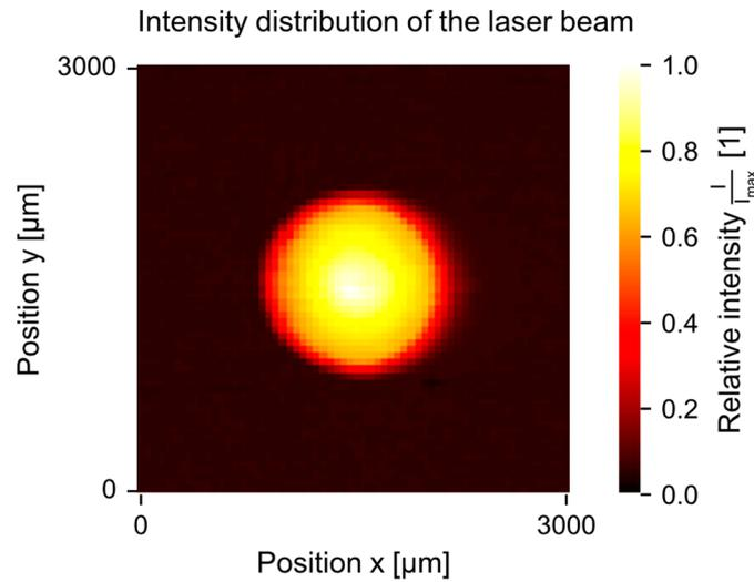
**Figure 3.** Intensity distribution of the laser beam used for the experiments performed in this work. The beam diameter according to the second-moment width is 1.2 mm.
