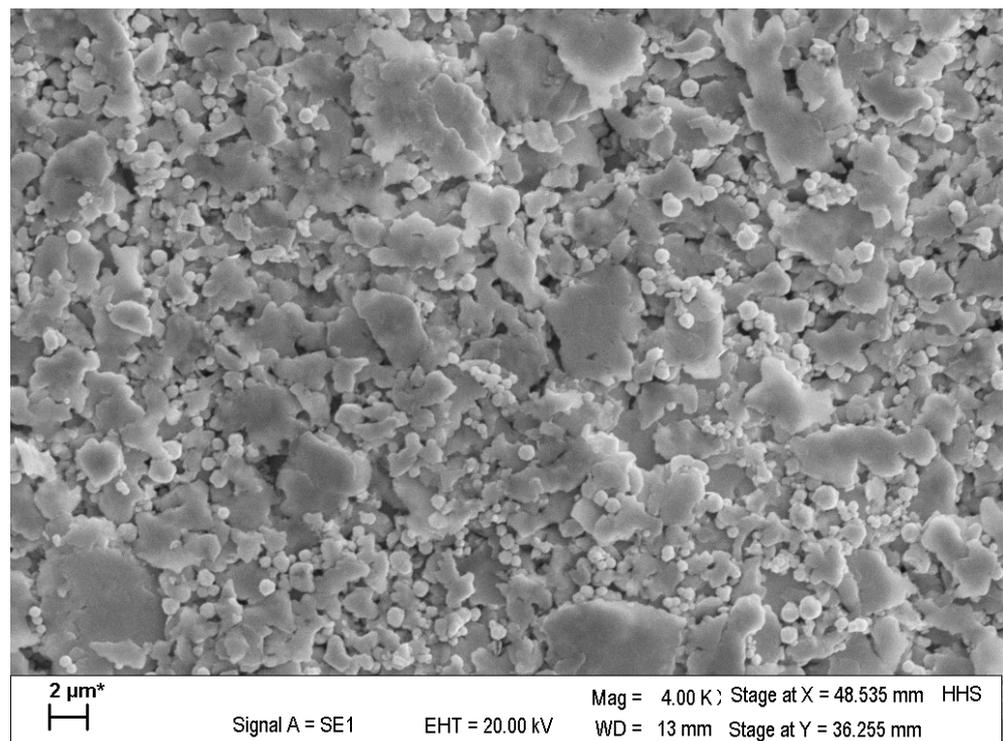
**Figure 1.** Scanning electron microscope (SEM) picture of the silver flakes used in the paste. The paste consists of small, almost spherical flakes, as well as large irregularly shaped flakes. All flakes consist of pure silver. For sample preparation, the components of the paste were separated using a centrifuge. The remaining flakes then were deposited onto a silicon wafer for SEM characterization.
