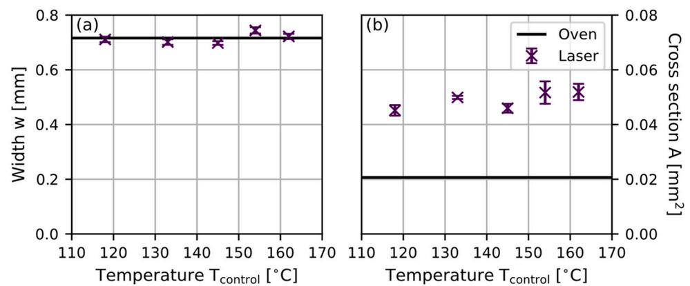
**Figure 10.** Results of the geometric characterization of the layers by LSM: (a) width of the traces as a function of the temperature, (b) calculated cross-section of the traces as a function of the temperature.
