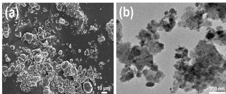
**Figure 1.** (a) SEM graph of PTFE powder and (b) TEM graph of  $\text{Cu}_2\text{O}$  nanoparticles.
