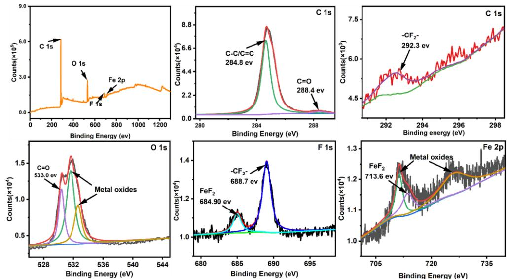
**Figure 9.** XPS spectra of the steel surface sliding against EP/1.5Cu<sub>2</sub>O/15PTFE.
