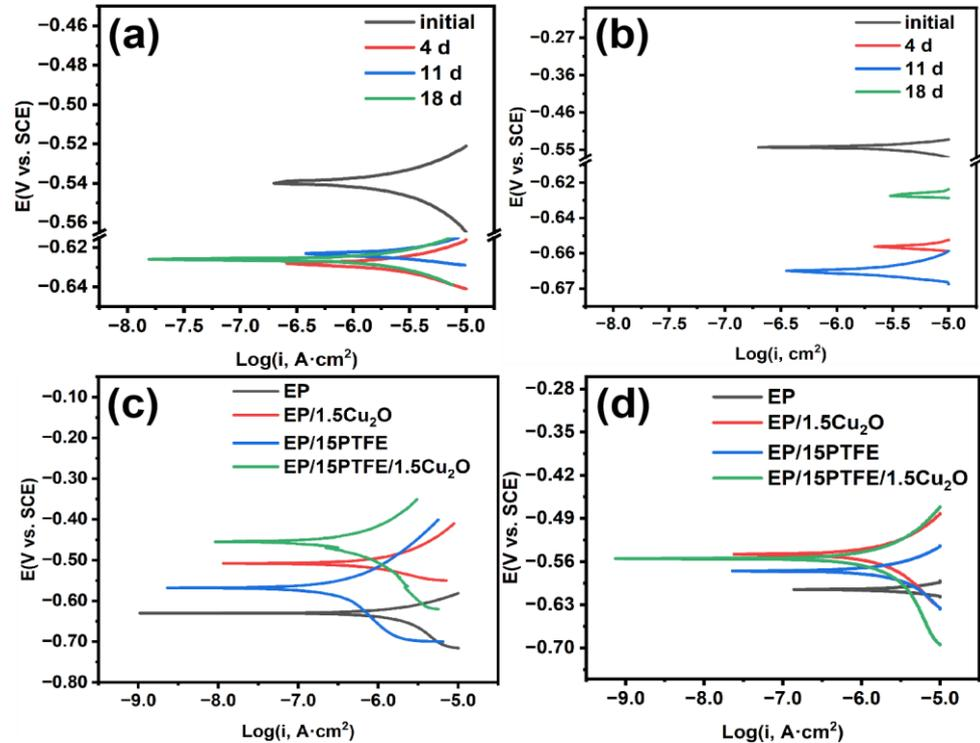
Figure 3. Potentiodynamic polarization curves of the Q20 steel (a,b) and the coatings (c,d) after being immersed in sterile (a,c) and SRB mediums (b,d) for 18 days.
