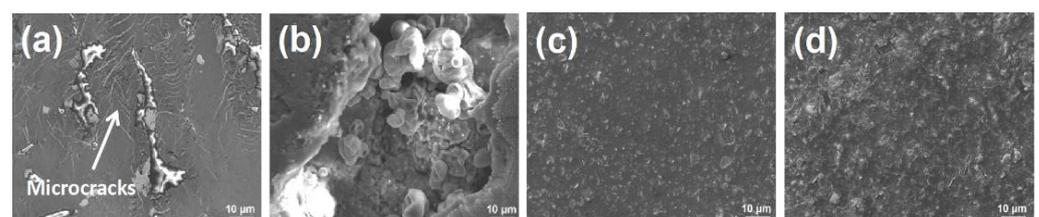
**Figure 6.** SEM images of EP in (a) sterile and (b) SRB medium for 18 days; SEM images of EP/1.5 $\text{Cu}_2\text{O}$ /15PTFE in the (c) sterile and (d) SRB medium for 18 days.
