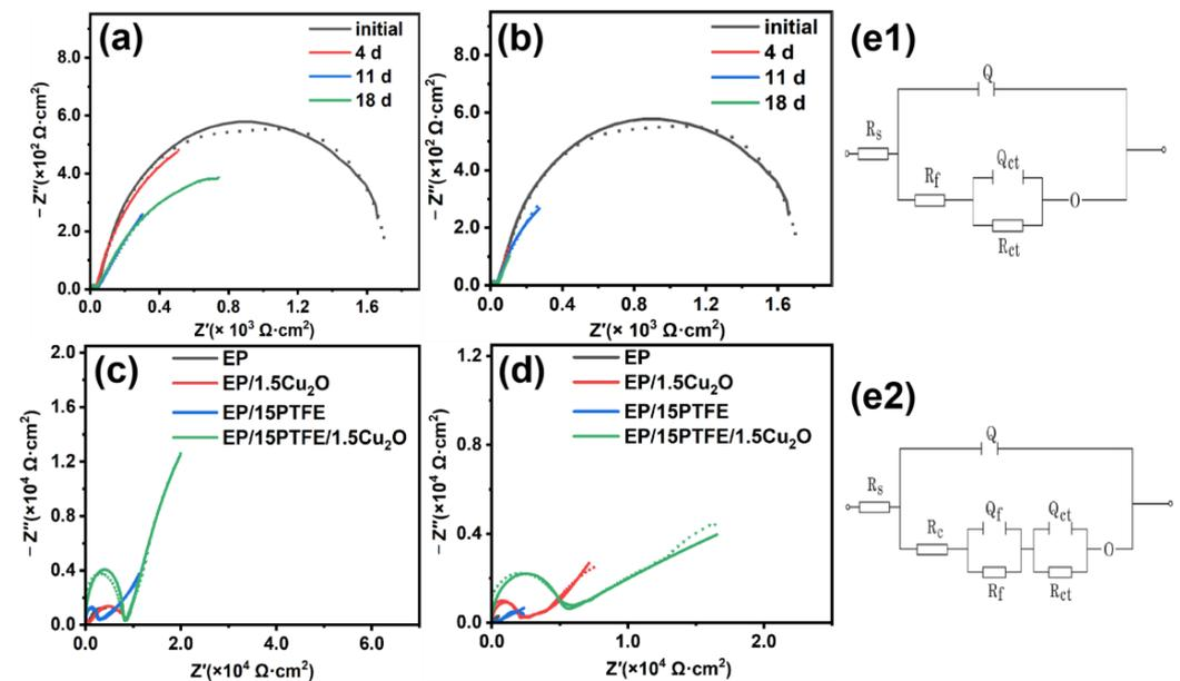
**Figure 2.** Nyquist plots of Q20 steel after immersion in sterile (a) and SRB mediums (b); Nyquist plots of coatings after immersion in sterile (c) and SRB mediums (d); equivalent circuit models for Q20 steel (e1) and coatings (e2).
