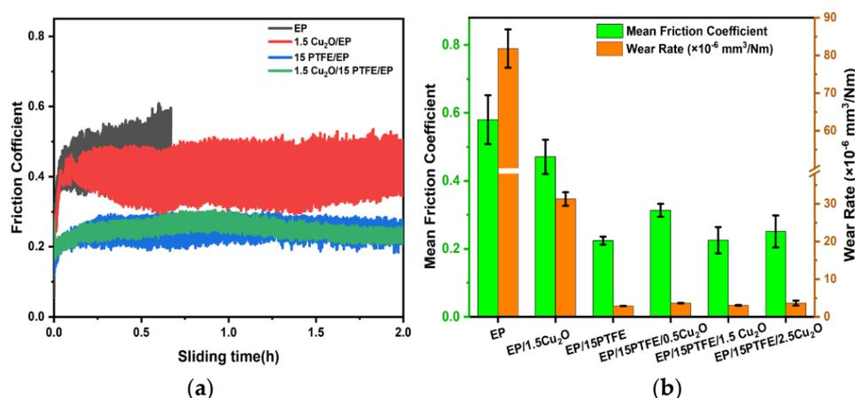
**Figure 7.** (a) Evolutions of friction coefficients of EP, EP/1.5Cu<sub>2</sub>O, EP/15PTFE and EP/1.5Cu<sub>2</sub>O/15PTFE; (b) mean friction coefficients and specific wear rates of the coatings investigated.
