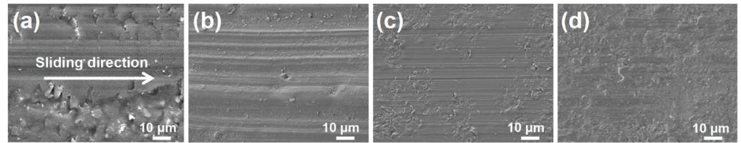
**Figure 8.** SEM graphs of worn surfaces of EP (a), EP/1.5Cu<sub>2</sub>O (b), EP/15PTFE (c) and EP/1.5Cu<sub>2</sub>O/15PTFE (d) sliding against the steel surface in water lubrication. Arrows indicate the sliding direction.
