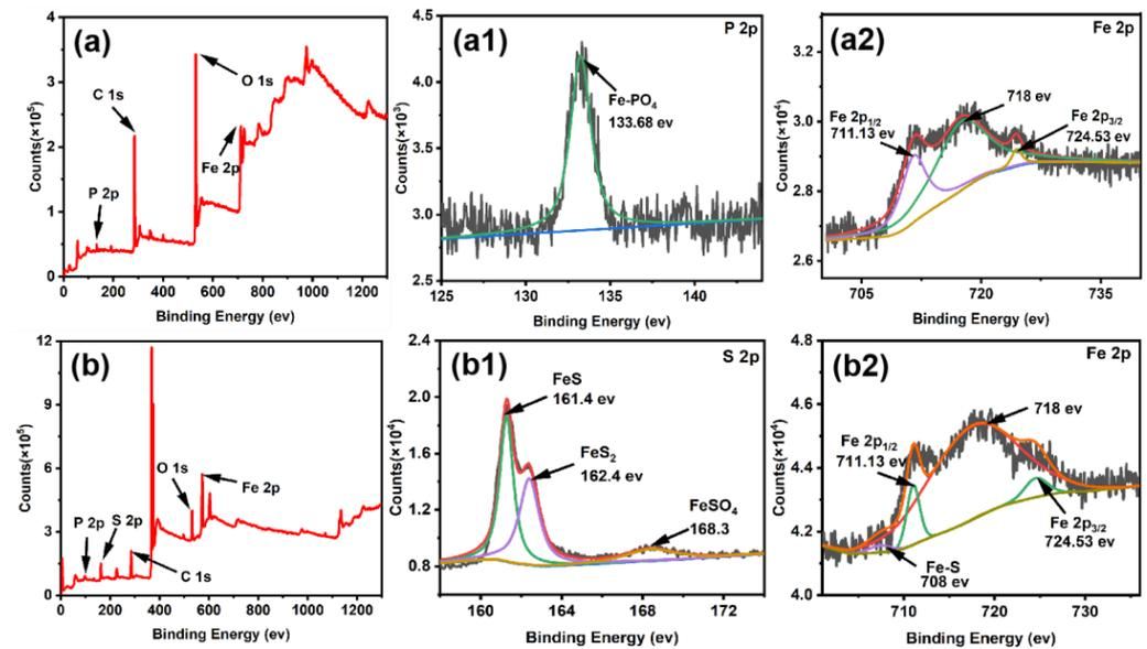
**Figure 5.** XPS spectra of Q20 steel surfaces after being immersed in the sterile medium (a,a1,a2) and the SRB medium (b,b1,b2) for 18 days.
