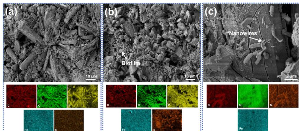
**Figure 4.** SEM graphs and EDS elemental maps of carbon steel surfaces after being immersed in the sterile medium (a) and the SRB medium (b,c) for 18 days.
