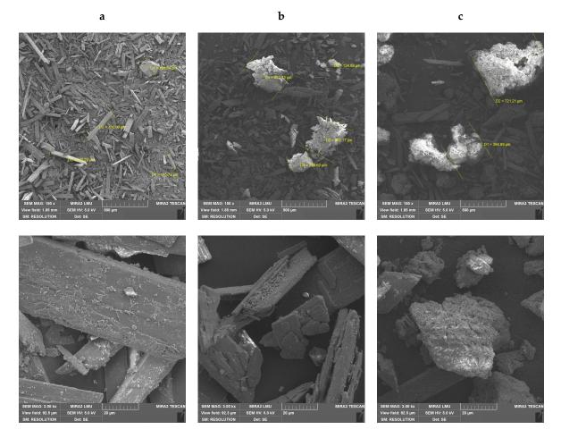
Figure 3. Morphology of the PGs particles. (a)—PG<sub>Bel</sub>; (b)—PG<sub>Bal</sub>; (c)—PG<sub>Kin</sub>.
