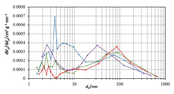
Figure 9. Pore volume distribution for binders, based on: --- NG; --- PG<sub>Bel</sub>; --- PG<sub>Bal</sub>; --- PG<sub>Kin</sub>.
