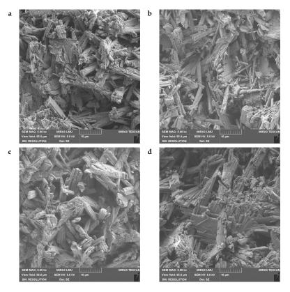
Figure 10. Morphology of the binders based on: (a)—PG<sub>Bel</sub>; (b)—PG<sub>Bal</sub>; (c)—PG<sub>Bal</sub>; (d)—NG.
