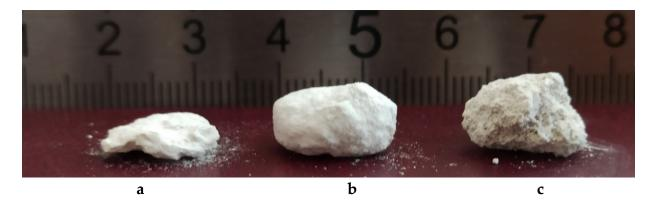
Figure 5. PG conglomerates with a size greater than 10 mm. (a)—PG<sub>Bel</sub>; (b)—PG<sub>Bal</sub>; (c)—PG<sub>Kin</sub>.
