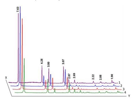
Figure 1. XRD-diagram of PGs and NG. --- NG (1); --- PG<sub>Bel</sub> (2); --- PG<sub>Bal</sub> (3); --- PG<sub>Kin</sub> (4).
