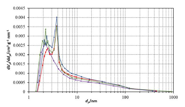
Figure 7. Pore size distribution of PGs and NG. — NaG; — PG<sub>Bel</sub>; — PG<sub>Bal</sub>; — PG<sub>Kin</sub>.
