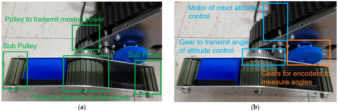
Figure 4. Unit for angle adjustment of undercarriage mechanism: (a) Parts related to belt power transmission; (b) Parts related to gear power transmission.
