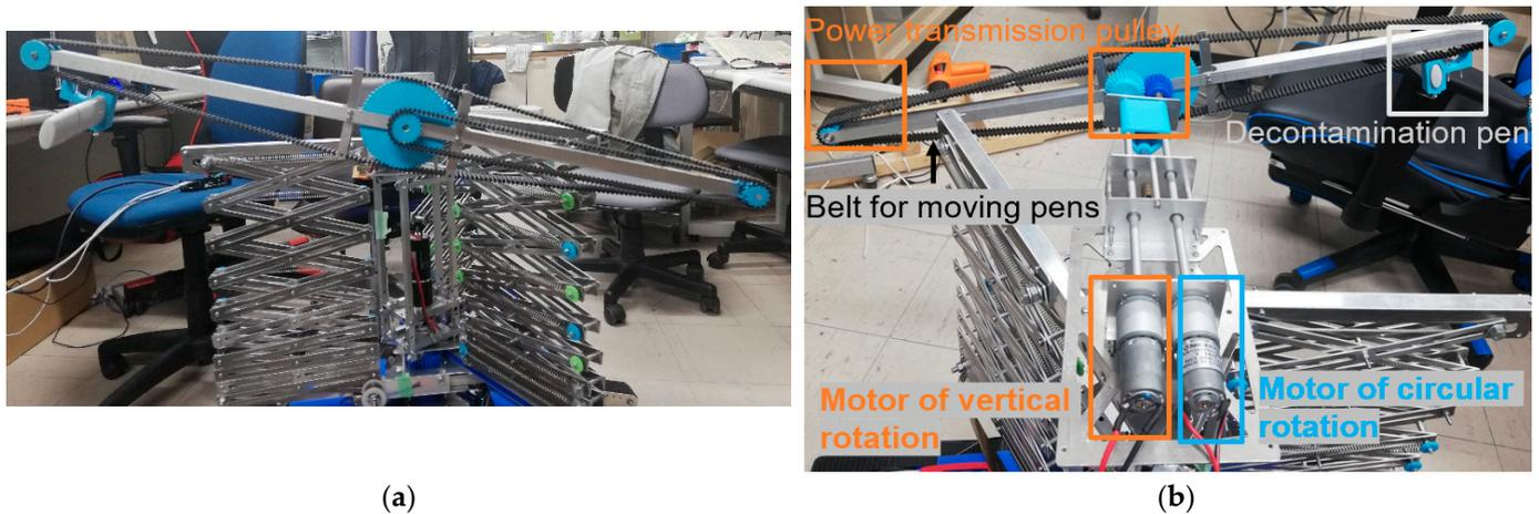
Figure 9. Decontamination mechanism: (a) Decontamination mechanism viewed from the front; (b) Decontamination mechanism viewed from behind at an angle.
