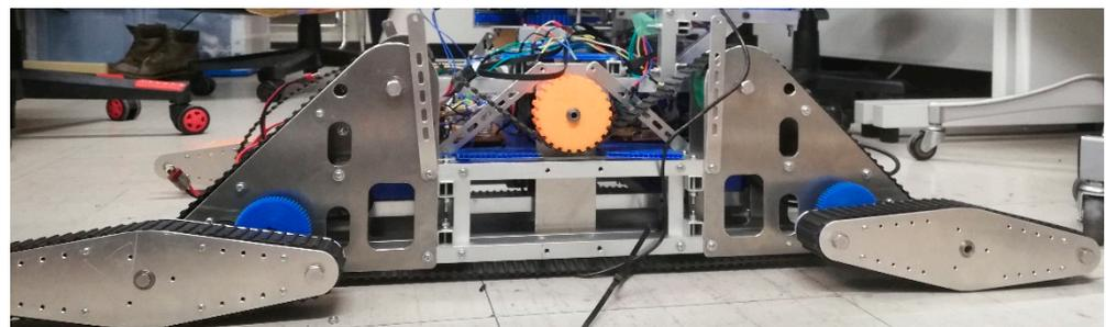
**Figure 3.** Undercarriage mechanism viewed from the side.
