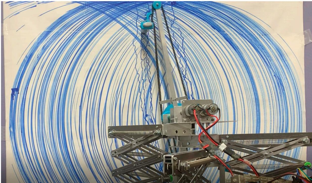
Figure 25. Decontamination by vertical rotation orbit of decontamination mechanism.
