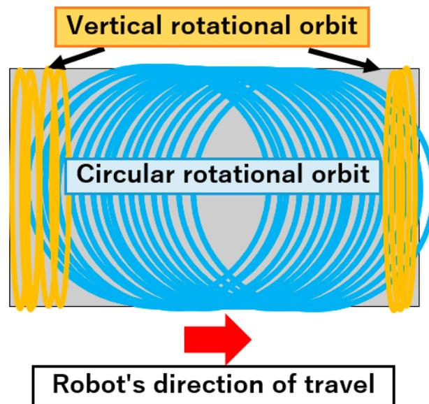
Figure 10. Diagram of decontamination method.
