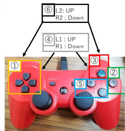
Figure 15. Controllers used for maneuvering.
