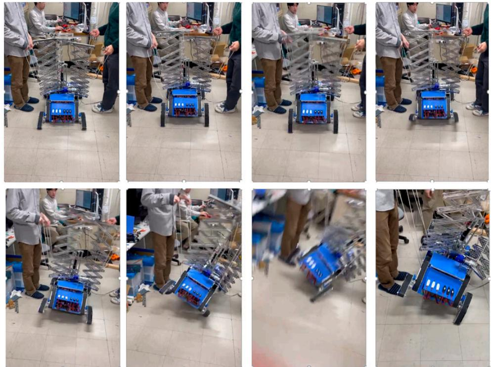
Figure 19. Result of robot operation before PID control.
