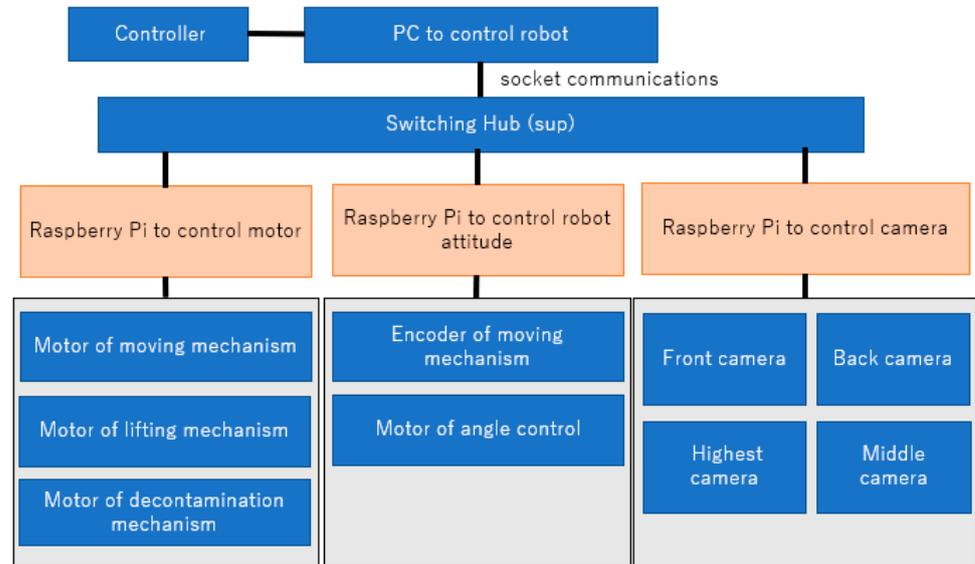
Figure 13. Control system connection diagram.
