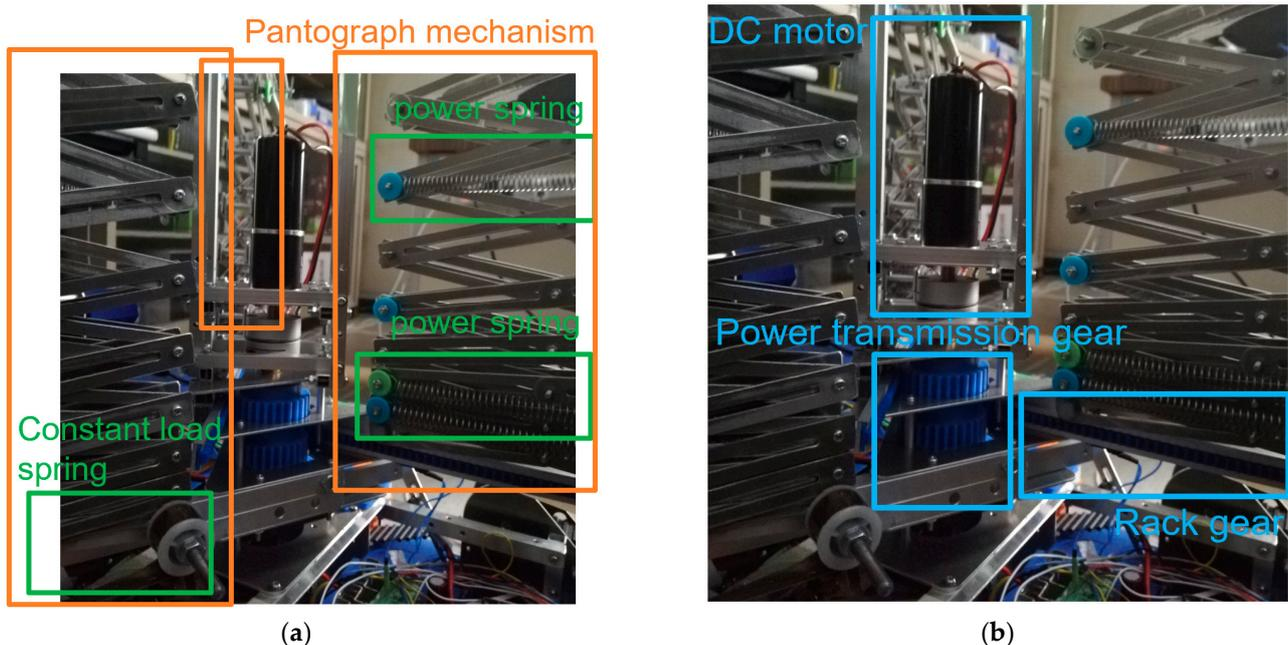
Figure 8. Central part of deployment mechanism: (a) Three pantograph mechanisms and supporting springs; (b) Location of power transmission components and motors.
