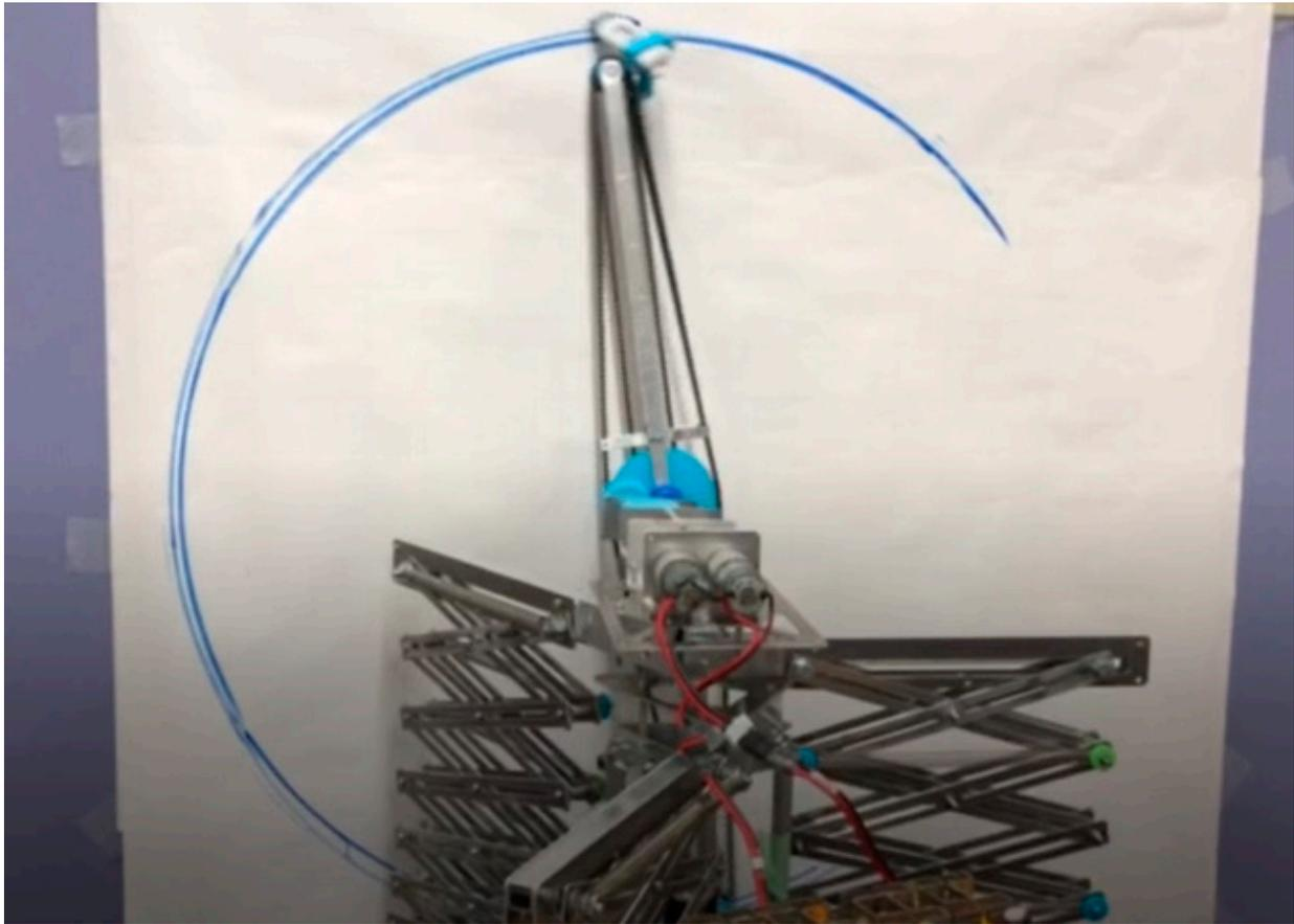
Figure 24. Decontamination by circular rotating orbit of decontamination mechanism.
