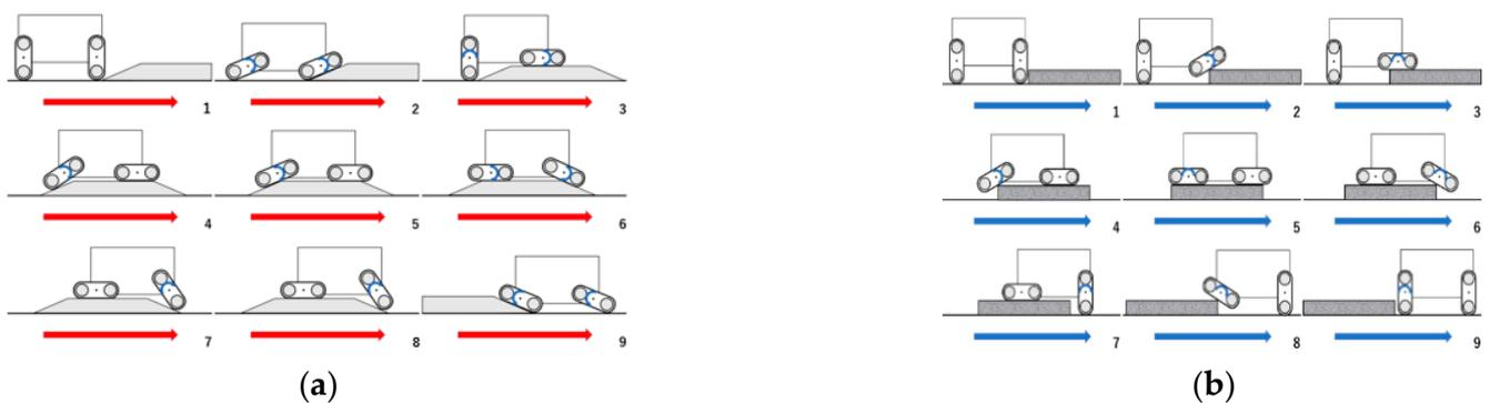
Figure 5. Imagery of Overcoming Slopes and Steps: (a) Overcoming a hill; (b) Overcoming Steps.
