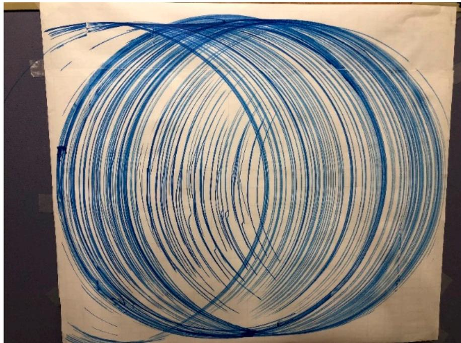
**Figure 26.** Results of decontamination by circular rotational orbit.
