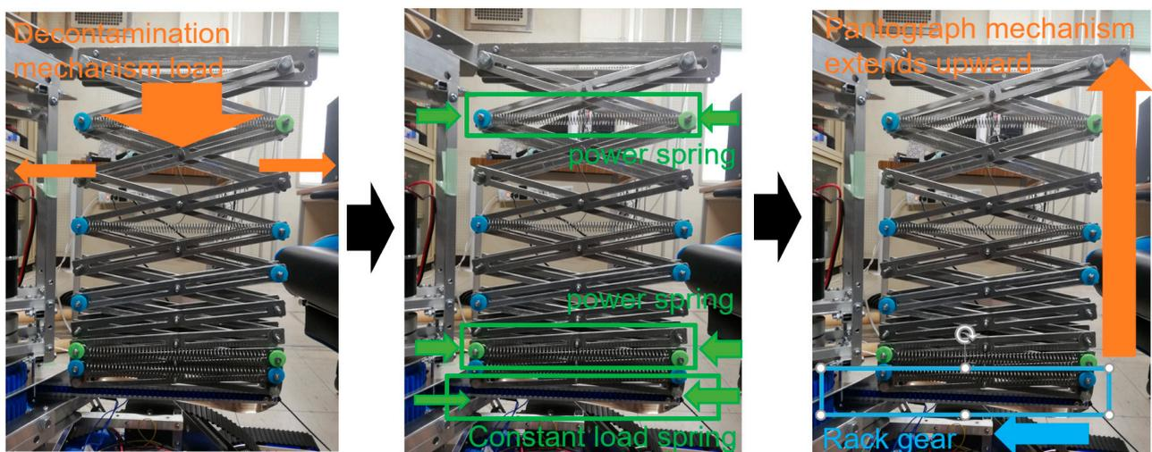
Figure 6. Operating Principle of Pantograph Mechanism for Elevating Mechanism.
